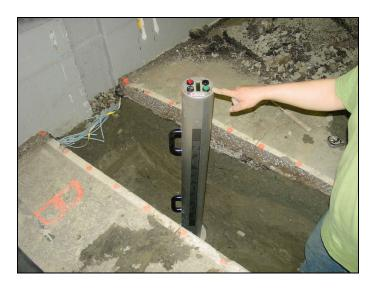
Figure 24. Portable falling weight deflectometer being used in the trenches.
