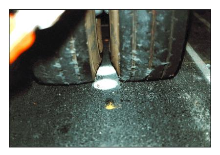
Figure 6. Location of test wheels over coil and stress cells.
