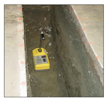
Figure 20. Nuclear gage density measurements in the trenches.
