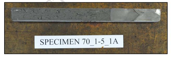
Figure 3.58: Specimen 70\_1-5\_1A fracture surface
