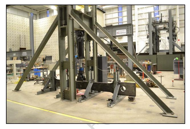
Figure 3.21: Axial test fatigue setup
