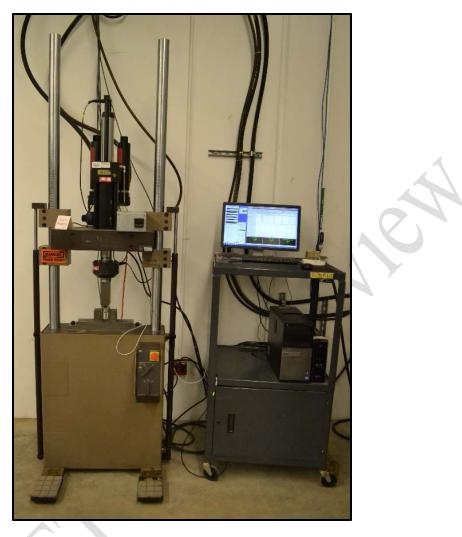
Figure 3.7: MTS Model 318.10 load frame setup
