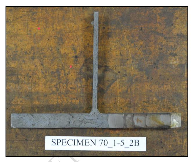
Figure 3.50: Specimen 70\_1-5\_2B fracture surface
