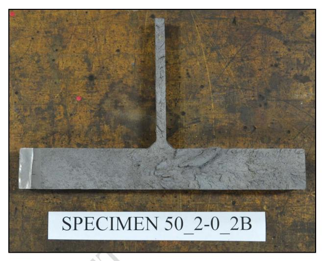
Figure 3.41: Specimen 50\_2-0\_2B fracture surface
