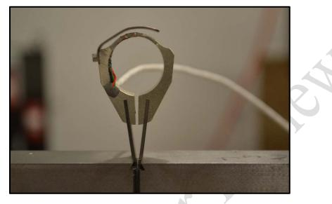
Figure 3.12: 0.25 in. displacement gage
