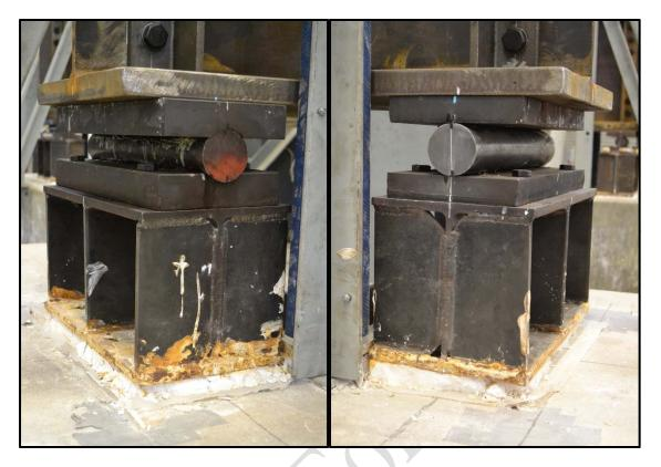
Figure 3.17: Pin bearing (left); Roller bearing (right)
