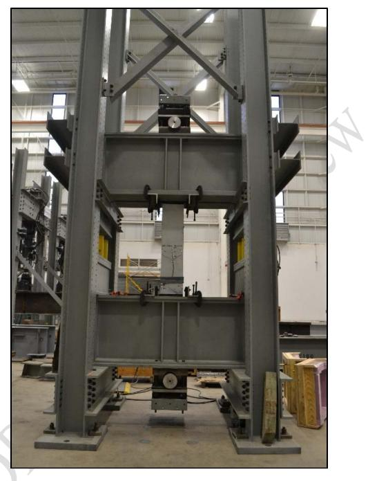
Figure 3.24: Axial test fracture setup
