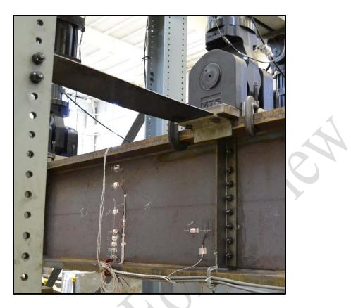
Figure 3.19: Lateral torsional buckling bracing
