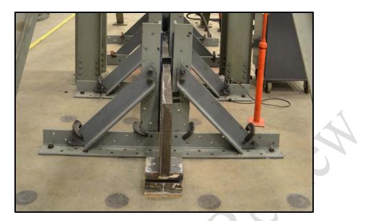
Figure 3.22: Axial fatigue test setup lateral bracing
