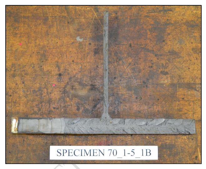
Figure 3.48: Specimen 70\_1-5\_1B fracture surface
