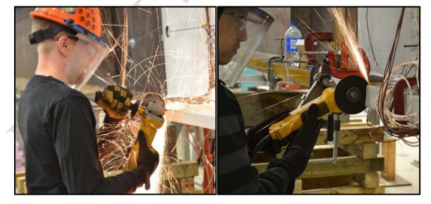
Figure 3.26: Straight notching (left); V-notching (right)
