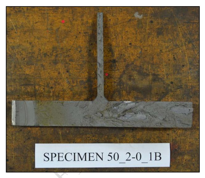
Figure 3.39: Specimen 50\_2-0\_1B fracture surface
