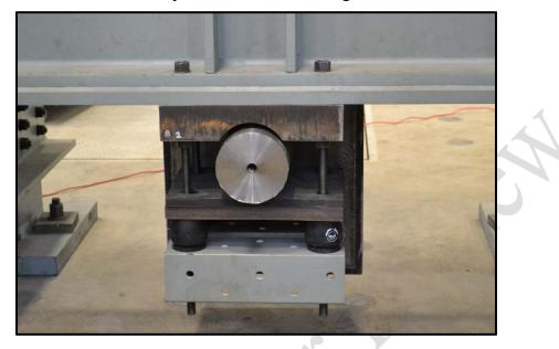
Figure 3.25: Axial load frame pin connection
