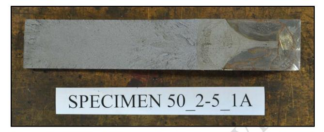
Figure 3.56: Specimen 50\_2-5\_1A fracture surface
