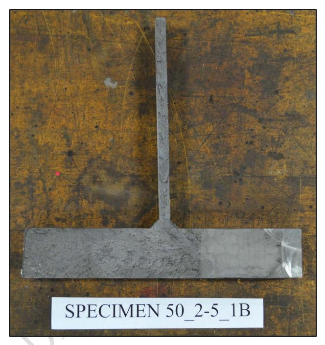
Figure 3.44: Specimen 50\_2-5\_1B fracture surface
