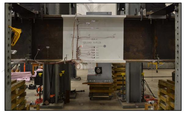
Figure 3.30: Example bending specimen instrumentation layout
