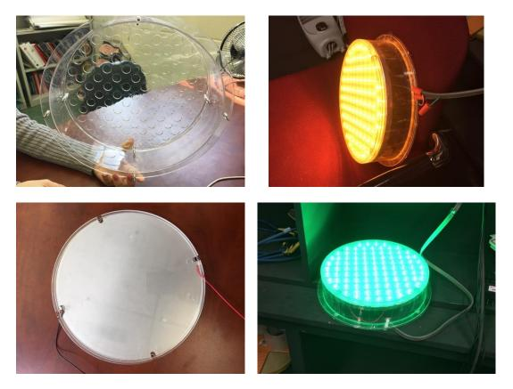
**Figure 1** Three samples the finalized design of the new housing of the fully working prototype signals of Type 1, modelled in the factory of Eco Molding. Each sample includes three plastic parts: the whole-piece of new housing that accommodate 96 small Fresnel lenses for light collimation of individual LEDs, a cover for
