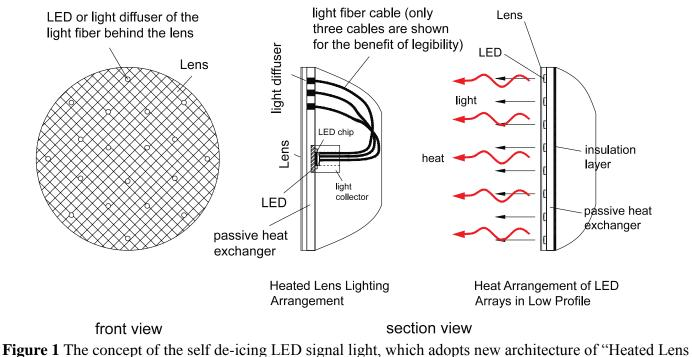
Lighting Arrangement" or "Heat Arrangement of LED Arrays in Low Profile"
