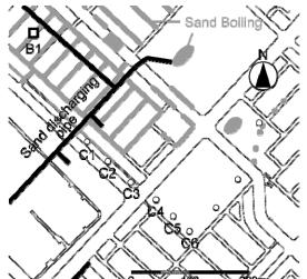
Figure 6. Mihama-ward site showing CPT locations, sand discharging pipe, and sand boiling traces (Sekiguchi and Nakai, 2012).
