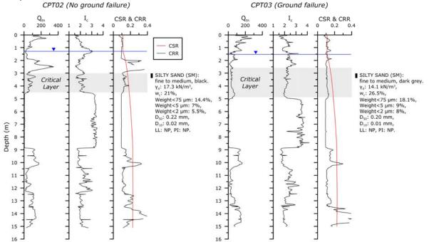
**Figure 2**. Normalized CPT resistance  $(Q_m)$ , soil behavior type index  $(I_c)$ , cyclic stress ratio (CSR) and cyclic resistance ratio (CRR) profiles on the location of no ground failure and ground failure. Laboratory index test results from the samples retrieved by a CPT sampler are indicated.
