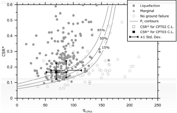
**Figure 3.** Liquefaction triggering database showing  $CSR^*$  vs.  $q_{cINcs}$  and  $CRR_{M7.5,\sigma'=1atm}$  for 15, 50, and 85% probabilities of liquefaction (after Boulanger and Idriss, 2014). Data points for critical layers and ±1 standard deviations of  $CSR^*$  and  $q_{cINcs}$  are shown for no ground failure (CPT02) and ground failure (CPT03) locations at example site in Urayasu, Japan.
