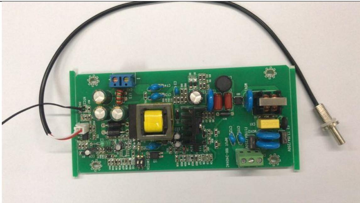
**Figure 4** The finalized design and a sample product of the new custom-made LED drivers, including one type for red light (input: 100-240 VAC, output: 0.6-1.1 A, max 30 W), and a second type for green/yellow light (input: 100-240 VAC, output: 0.5-0.8 A, max 30 W). Both types of LED drivers are integrated with a remote temperature sensor and an on/off switch for winter and summer modes.
