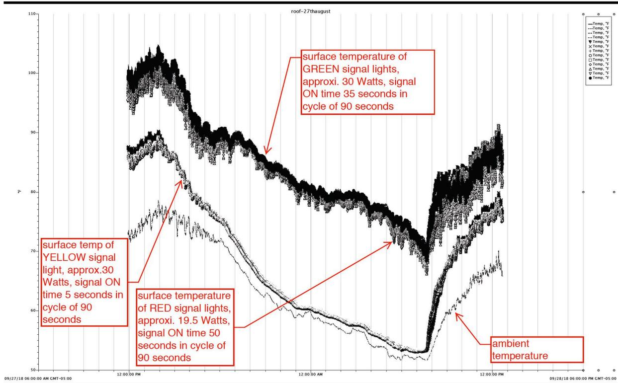
**Figure 2** A typical day portion of the test data recorded on Aug 27, showing surface temperature changes with ambient air temperature and solar heat gain in the morning.
