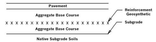
Figure 1: Base Course Reinforcement Using Geosynthetics
