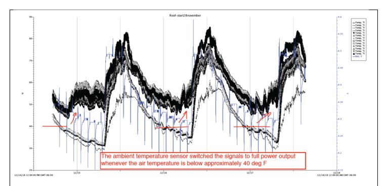
**Figure 3** The roof test data recorded in the snowy winter conditions, showing surface temperature jumped when the ambient air temperature was below 4 deg Celsius (39.2 deg Fahrenheit) as designed.
