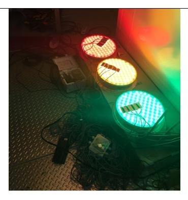
**Figure 4** The tests of the fourth generation of prototype signals in the cold room, to double check the switching performance of the ambient air temperature sensor attached to each signal.
