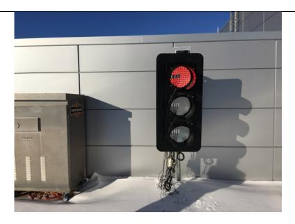
**Figure 2** In real-time snowy winter, the closed-course performance and reliability tests of the fully workin prototypes mounted on the roof of M2SEC building. The roof tests will be continuously conducted in 2019 with necessary real-time adjustments.
