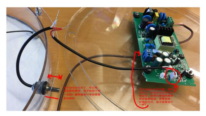
**Figure 5** The switching temperature sensor attached to each signal has some problems of wiring, need improvement.
