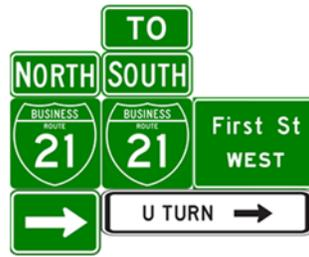
FIGURE 7. DIRECTIONAL ASSEMBLY RECOMMENDED FOR MINOR APPROACHES.
