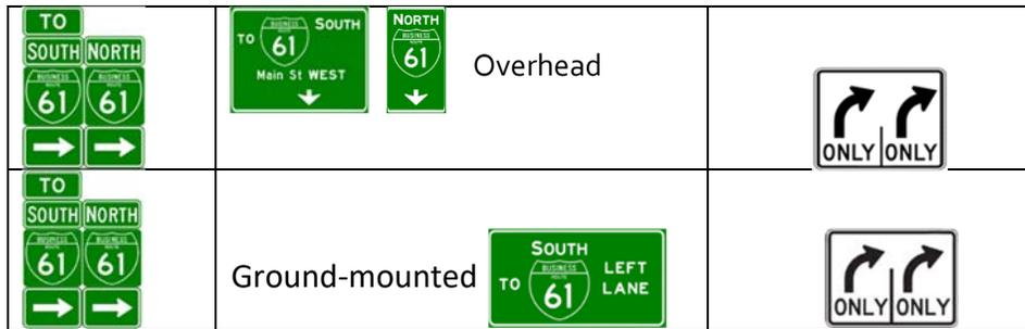
FIGURE 9. EXAMPLES OF TWO OF THE FOUR SIGN SEQUENCES TESTED FOR MULTI-LANE MINOR APPROACHES.
