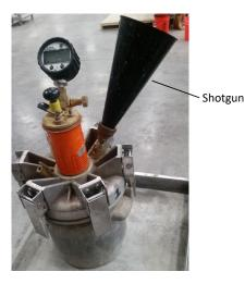
Figure 2.4.2 – A funnel and threaded tube that allows water to be continuously added to the bottom chamber while filling.
