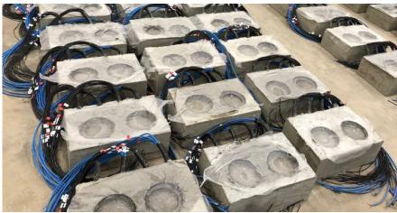
Figure 3.4.4 – An overview of the mortar samples being prepared and also surrounded by the concrete cover and ready for the instrumentation box.
