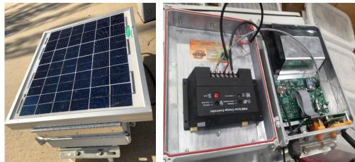
Figure 3.4.5. Instrument box with solar panel
