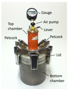
Figure 2.1.1 – The device used to complete the SAM.
