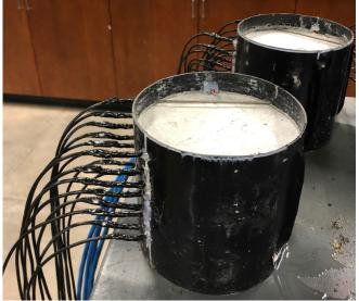
Figure 3.4.3. Mortar sample molds.
