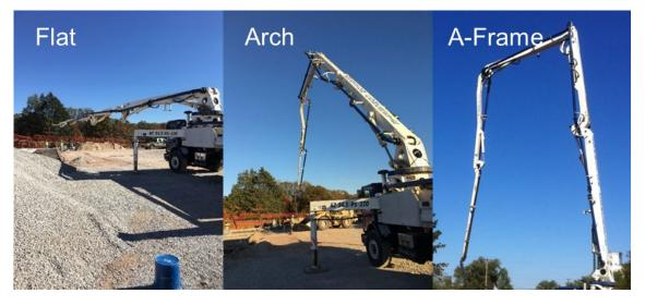
Figure 2.6.1. The flat, arch, and A-Frame orientations of the concrete pump.
