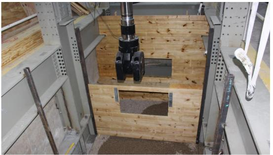
Figure A 2: Partition Walls Installation
