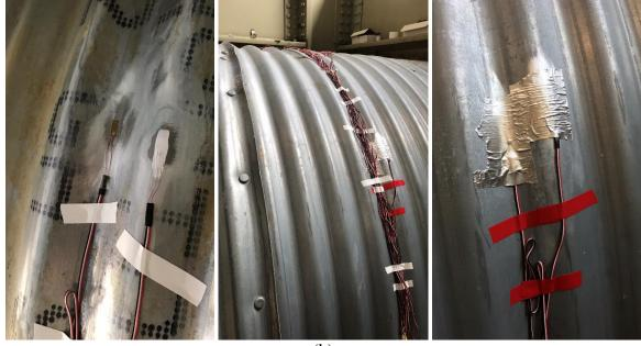
(b) Figure A 10, (a) and (b): Attaching Strain Gauges
