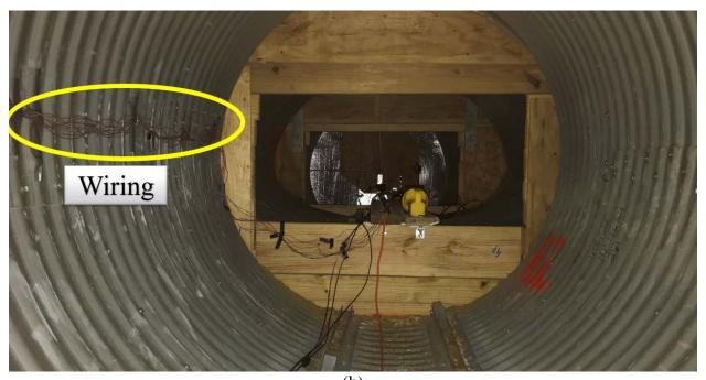
(b) Figure A 15, (a) and (b): Partition Walls Opening and Wiring
