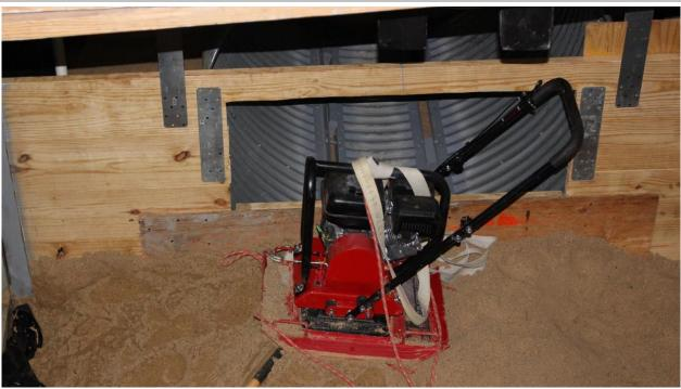
Figure A5: Vibratory Plate Compactor
