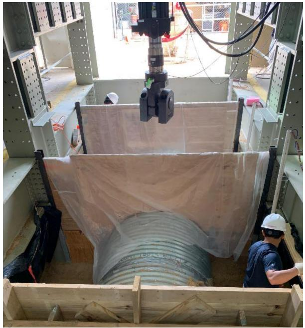
Figure A 17: Completion the Installation of Partition Walls and Placing Plastic Sheets
