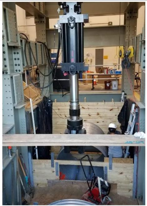
(b) Figure A 7, (a) and (b): Placing Circular CMPs
