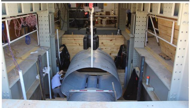
Figure A 13: Placing Arch CMP
