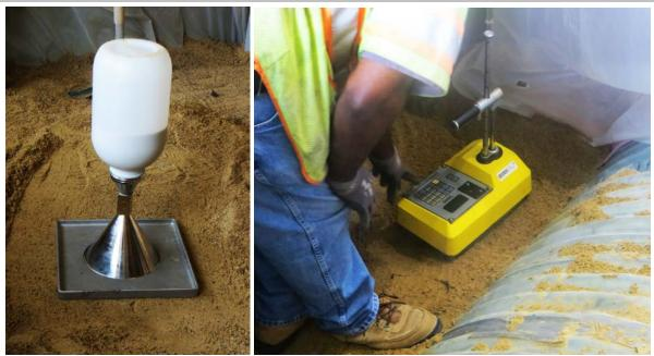
Figure A 18: Sand Cone Test and Nuclear Density Measurement
