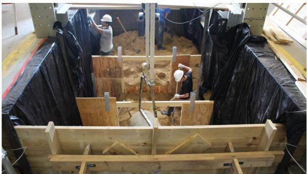
Figure A 6: Plastic Sheets Installation
