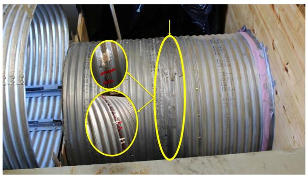
Figure A 14: Physical Protection of Strain Gauges by Aluminum Tape
