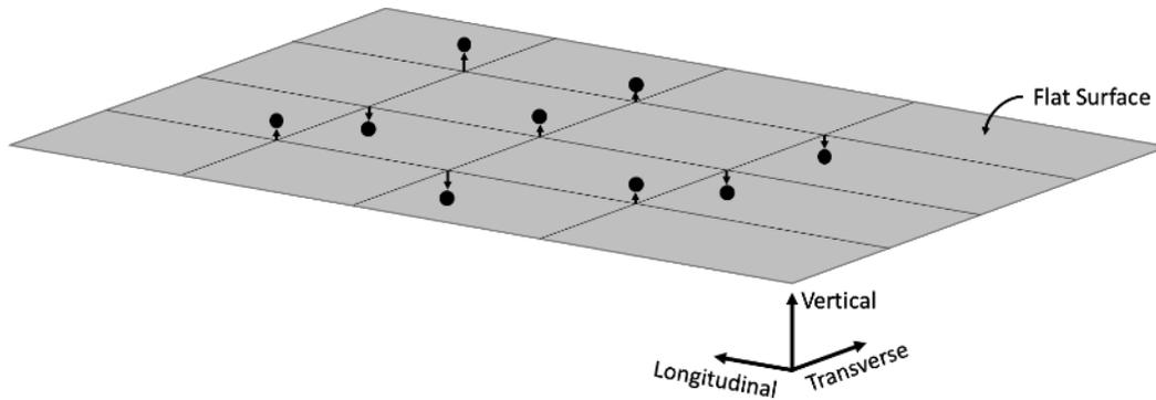
Figure 13. Deviation of vertical measurement heights from a flat surface.
