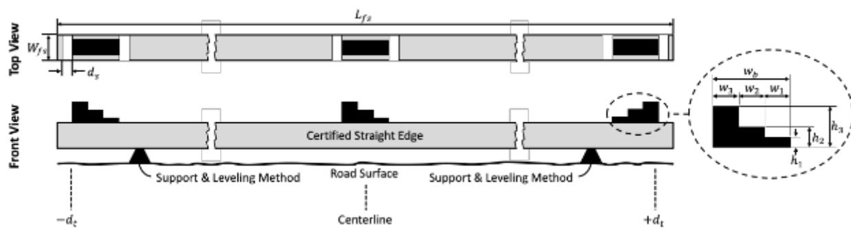
Figure 58. Detailed schematic of the layout of the gauge blocks on the leveled straight edge.
