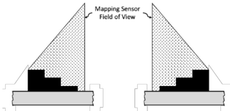
Figure 33. Orientation of a stair-stepped gauge block to best align with the field of view of the mapping sensor.
