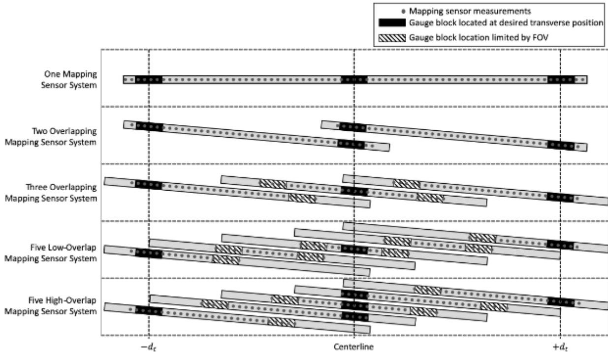
Figure 30. Alignment of the straight edge with the mapping sensor measurement path.
