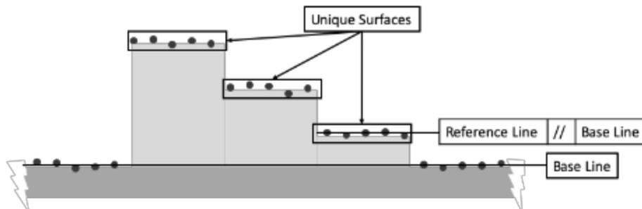
Figure 34. Definition of a base line corresponding to measurements located on the straight edge and a parallel reference line which spans a selected reference set of measurements (e.g. bottom step of the gauge block).
