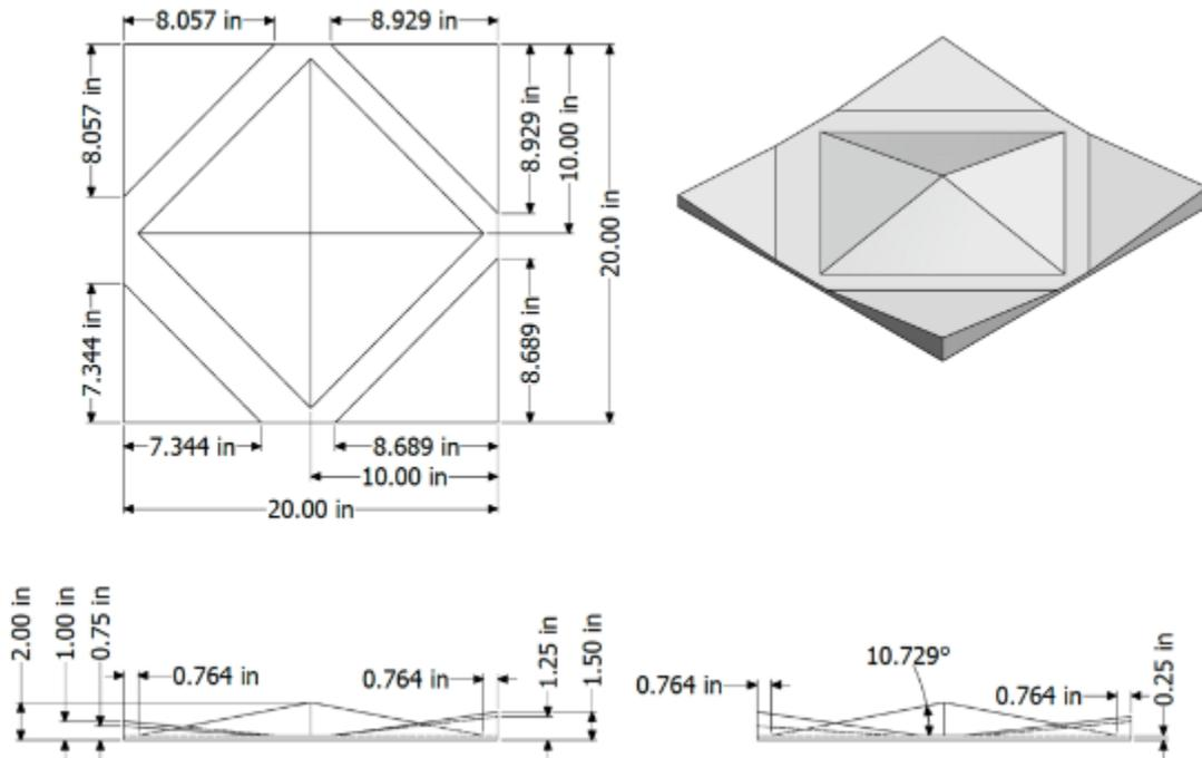
Figure 69. Dimensioned drawing of the reference object used in the navigation drift assessment during the second equipment rodeo.
