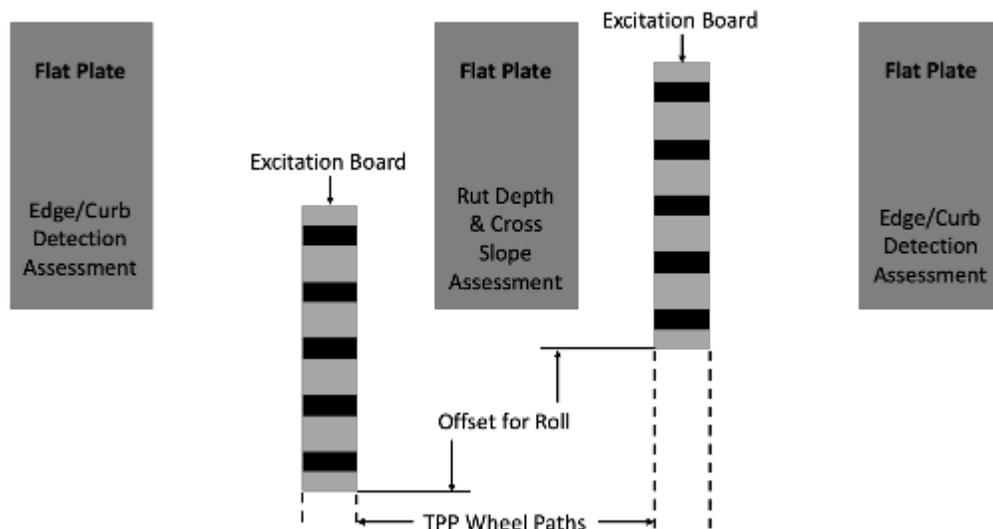
Figure 20. Layout of the two offset excitation boards and flat plates for the body motion cancelation assessment.
