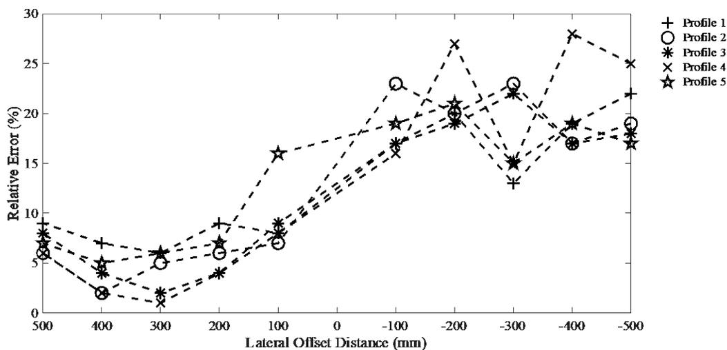
Figure 14. Relative error as a function of lateral offset for a non-symmetrical rut shape.<sup>(17)</sup>
