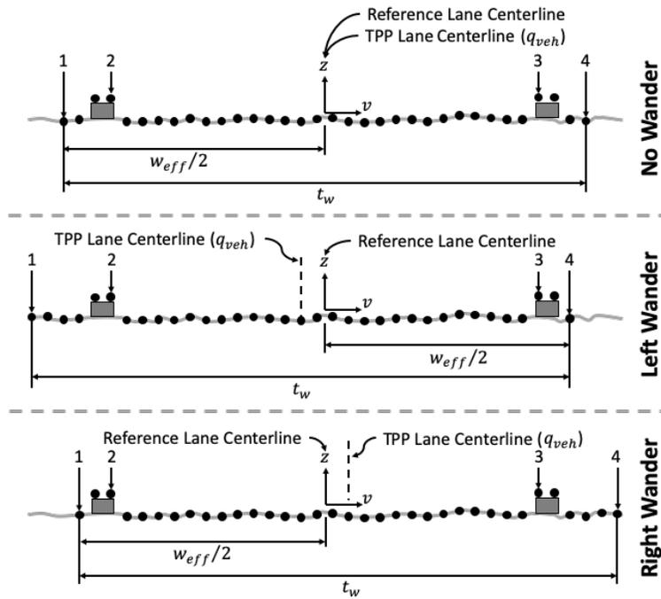
Figure 47. Representation of vehicle transverse wander in a single transverse profile.
