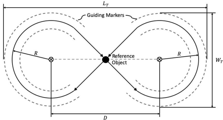
Figure 42. TPP drift assessment schematic.
