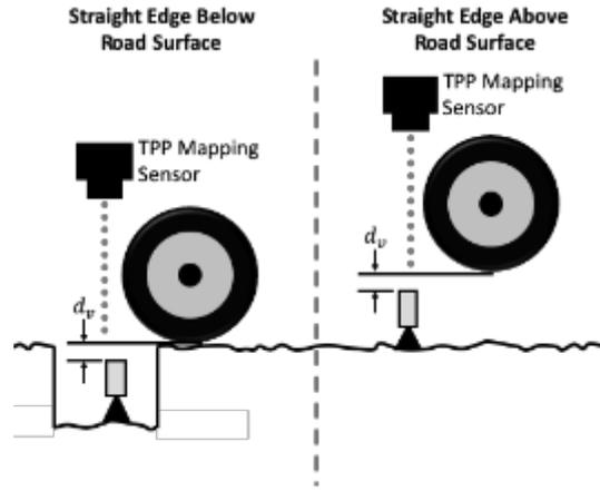
Figure 31. Elevation of the TPP, or depression of the straight edge, to ensure proper vertical positioning of the mapping sensor to the top of the straight edge.
