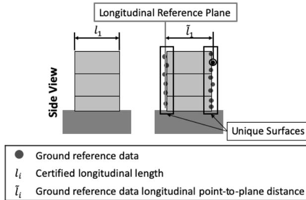
Figure 62. Identification of unique surfaces of a gauge block corresponding to longitudinal error measurement in the ground reference data point cloud, and example longitudinal point-to-plane distances for each unique surface set.
