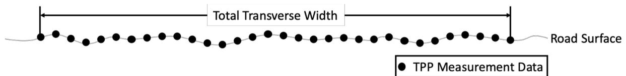
Figure 6. Total transverse width dimension for an individual transverse measurement profile.
