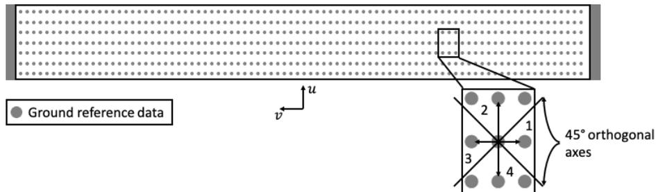
Figure 59. Illustration of four quadrants oriented with respect to the path coordinate system and identification of the nearest neighboring point in each respective quadrant.
