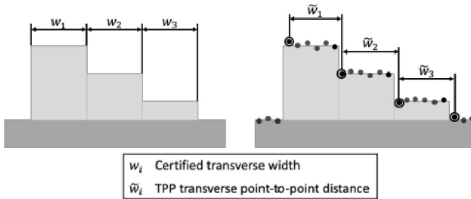
Figure 38. Example transverse point-to-point distances for a given horizontal gauge block surface.
