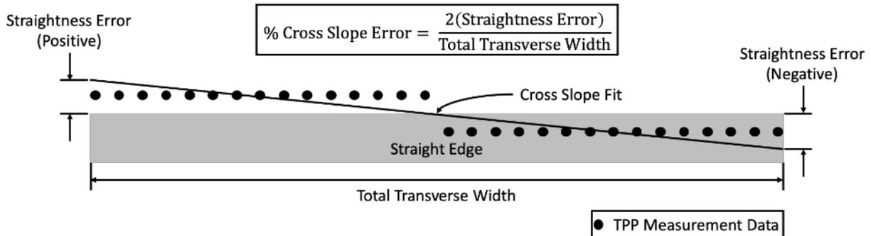
Figure 12. Worst case straightness error stack-up for determining cross slope error.
