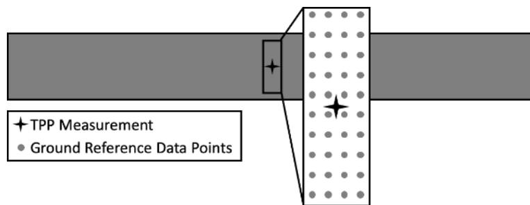
Figure 17. Identification of ground reference data points in the neighborhood of an individual TPP measurement of the road surface.
