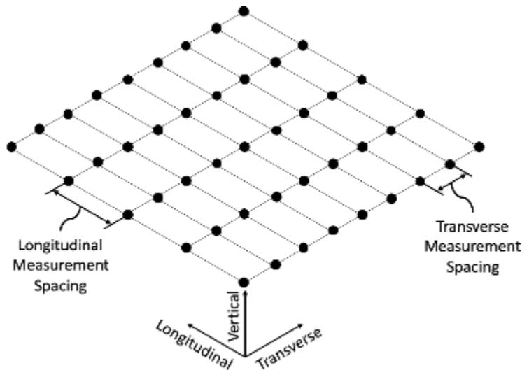
Figure 7. Illustration of transverse and longitudinal measurement spacing for a set of TPP measurements.
