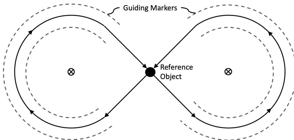
Figure 21. Figure-eight layout with a reference object placed at the center of the figure-eight to assess navigation drift.
