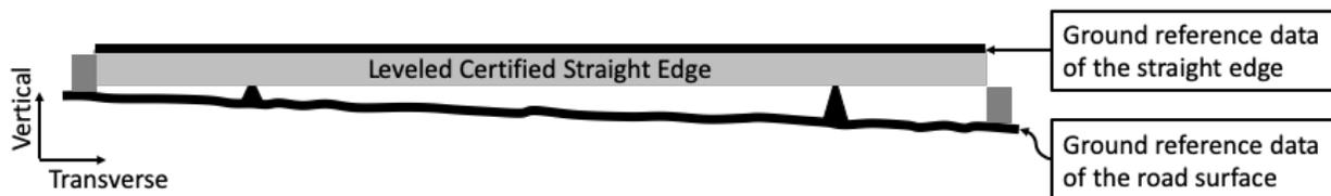
Figure 53. Proper orientation of the ground reference data, when viewed in the transverse-elevation plane, for calculation of cross slope.
