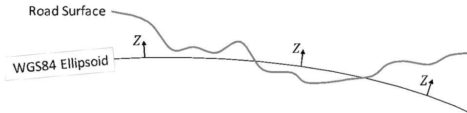
Figure 29. Representation of the vertical direction which is normal to the WGS84 Ellipsoid.
