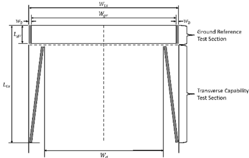
Figure 45. Schematic of the complete test site with the ground reference test section adjoining the transverse capability test section.
