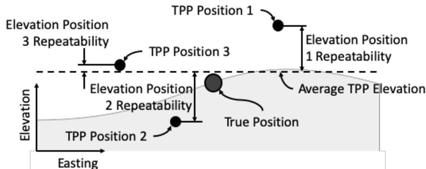
Figure 16. Elevation position repeatability for three example TPP reported locations of a stationary object (represented by the true position).
