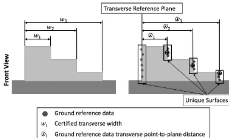
Figure 61. Identification of unique surfaces of a gauge block corresponding to transverse error measurement in the ground reference data point cloud, and example transverse point-to-plane distances for each unique surface set.
