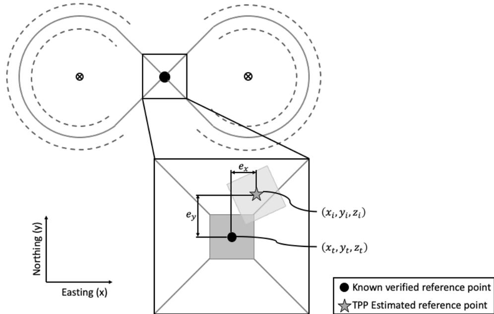
Figure 44. Illustration of the easting and northing position errors between the global position of the reference object and an estimated position of the object based on the TPP point cloud.
