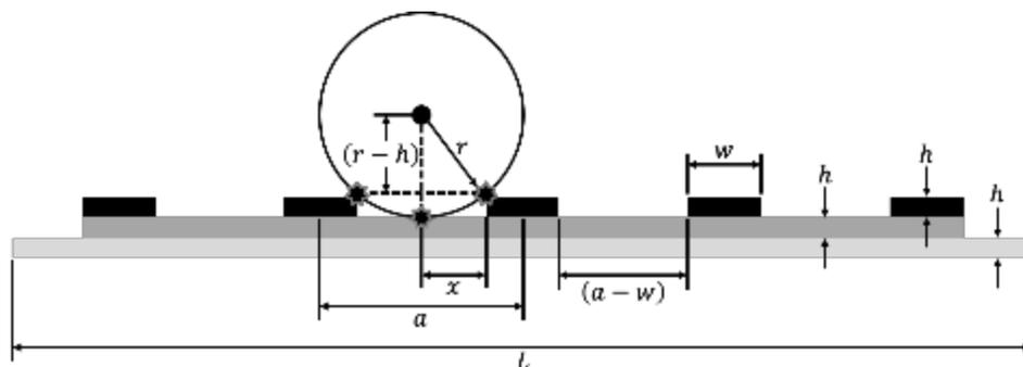
Figure 66. Dimensioned excitation board schematic with typical tire diameter represented by the black ring.
