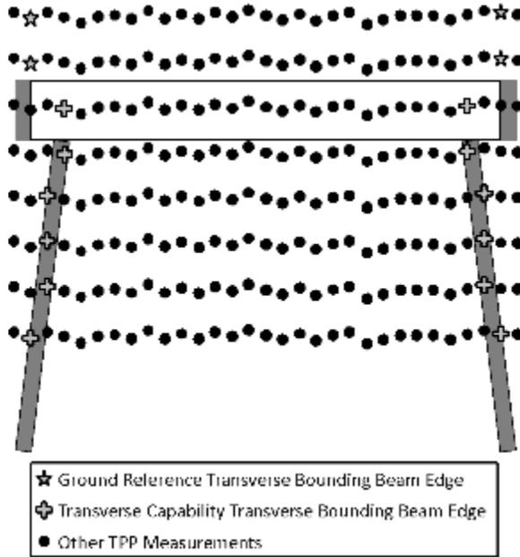
Figure 49. Transverse translation of the TPP dataset based on the best alignment of the ground reference transverse bounding beams.
