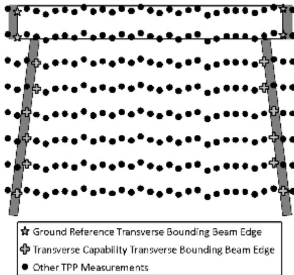
Figure 50. Longitudinal translation of the TPP dataset based on the best alignment of the angled bounding beams in the transverse capabilities test section.
