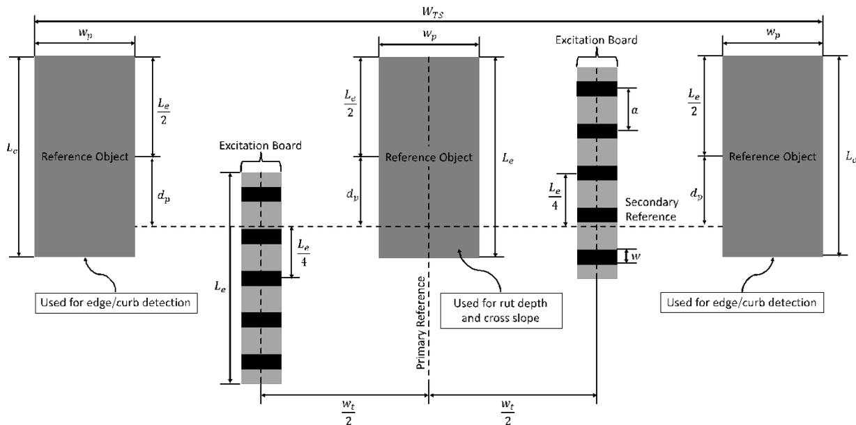
Figure 39. Vehicle motion compensation setup to induce primary ride and roll TPP harmonic.
