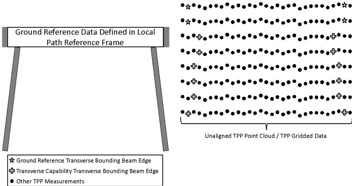
Figure 48. Identification of transverse bounding beam edges in the TPP dataset for the ground reference and transverse capabilities test section.
