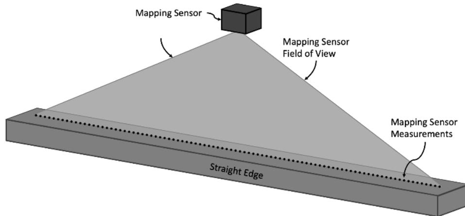
Figure 19. Mapping sensor centered over a leveled straight edge such that the field of view of the sensor is completely on the straight edge surface.
