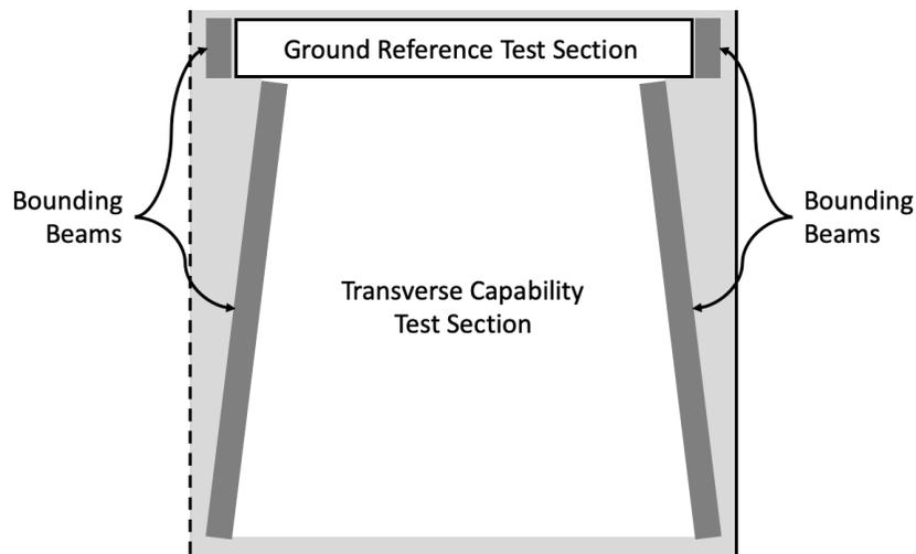
Figure 22. Layout of the transverse capability and ground reference test sections, defined by the bounding beams placed on the road surface.
