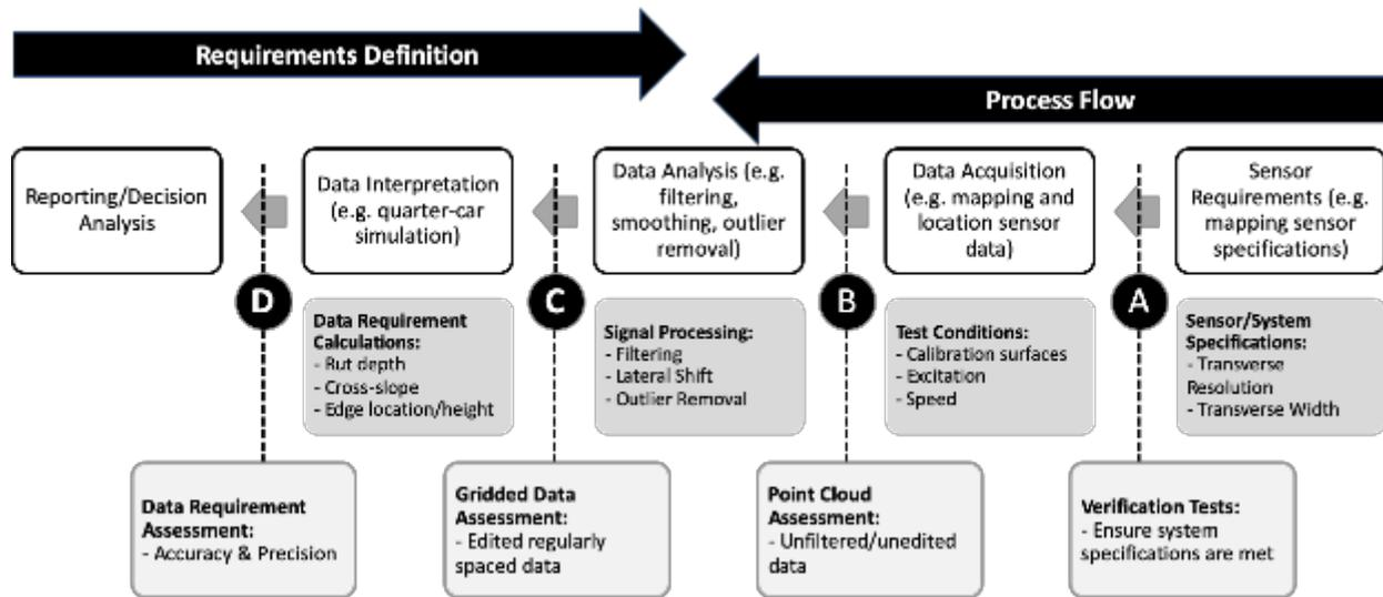
Figure 1. Layers of Assessment for Measurement of Transverse Profiles
