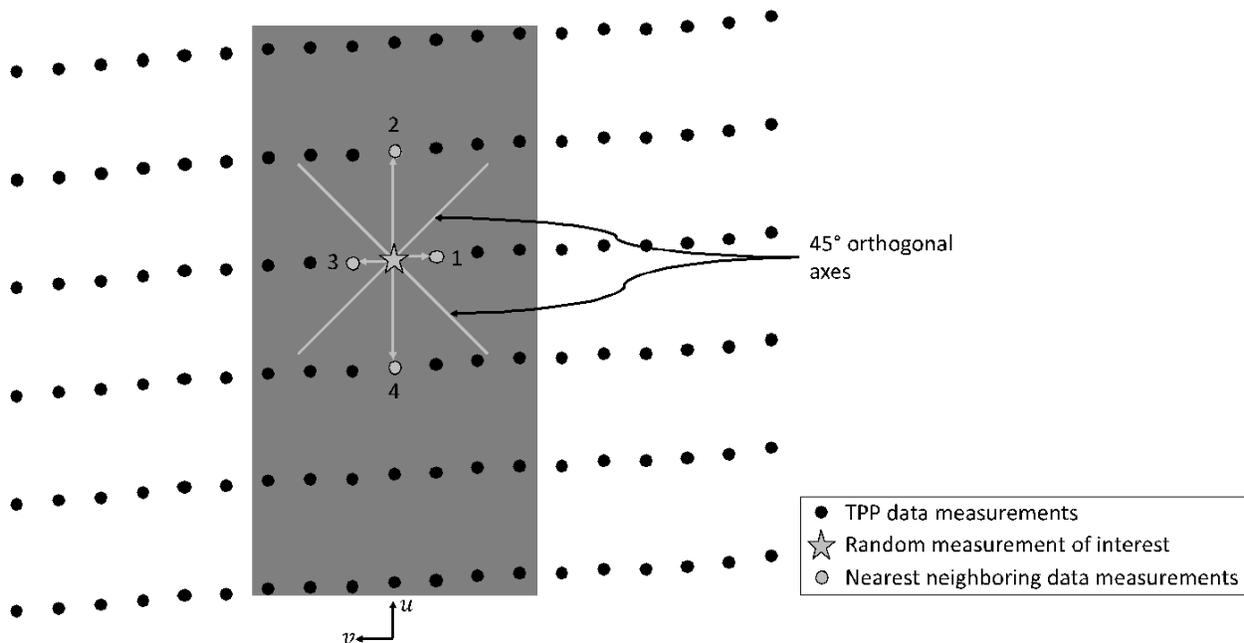
Figure 41. Illustration of four quadrants oriented with respect to the path coordinate system and identification of the nearest neighboring point in each respective quadrant.
