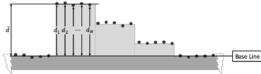
Figure 35. Representation of a nominal surface plane based on the average point-to-line distances for an individual gauge block surface.
