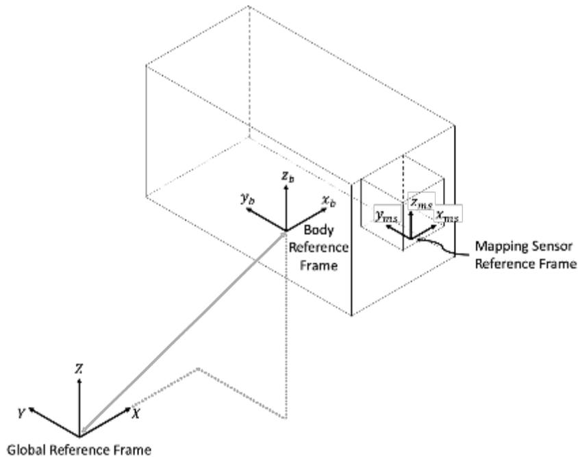
Figure 2. Relationship between global, body, and mapping sensor reference frames.
