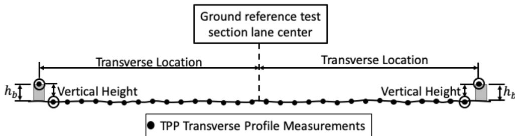
Figure 55. Identification of the vertical height and transverse location for the transverse bounding beams in the ground reference test section from the TPP transverse profile measurements.
