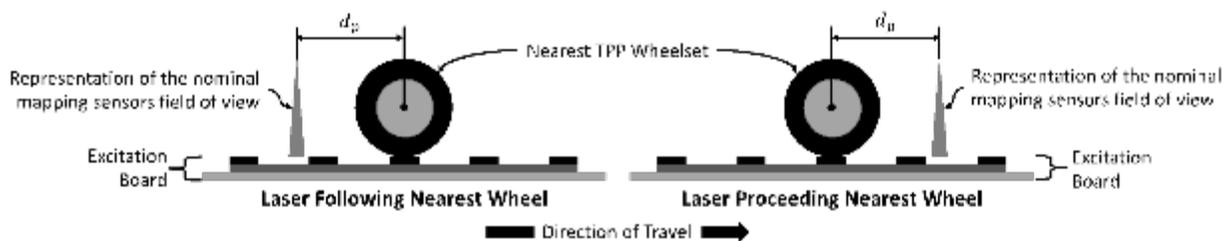
Figure 40. Determination of the plate offset based on the nominal mapping sensor offset from the nearest wheelset of the TPP.
