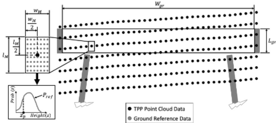
Figure 51. Ground reference rectangular region of interest to determine point cloud vertical error.
