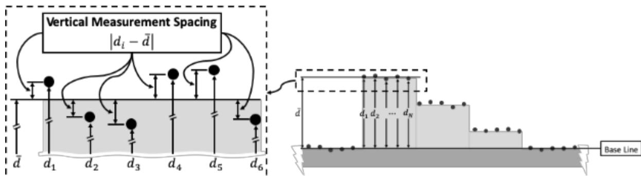
Figure 36. Illustration of vertical measurement spacing based on the absolute difference in the point-to-line distance of each measurement with the average point-to-line distance.
