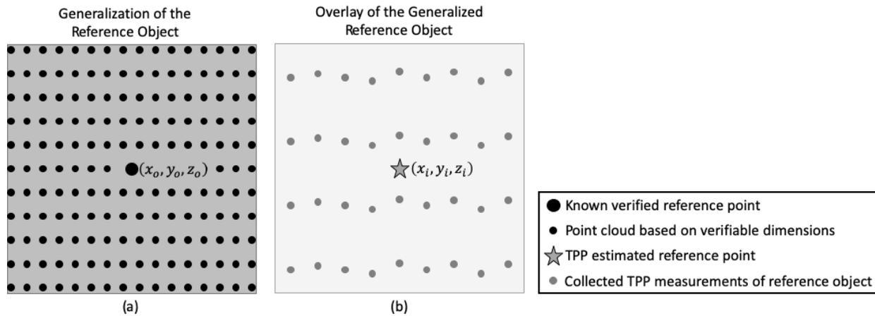
Figure 43. (a) Generalized reference object with reference point cloud based on verifiable dimensions which are referenced to the reference point ( , , and ). (b) Estimated location of the reference point based on the lowest distance error fit of the reference point cloud to the TPP point cloud measurements of the reference object.
