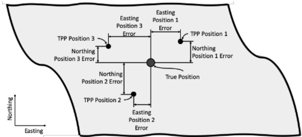
Figure 15. Northing and easting position error for three example TPP reported locations of a stationary object (represented by the true position).
