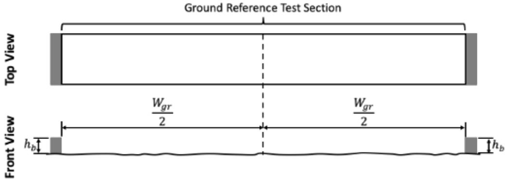
Figure 56. The curb transverse location is known based on the ground reference test section transverse width ( $W_{gr}$ ) and the height of the curbs are known based on the height of transverse bounding beams ( $h_b$ ).
