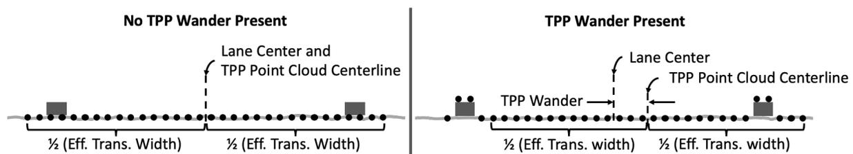
Figure 23. Effect of wander on the effective transverse width of the TPP.
