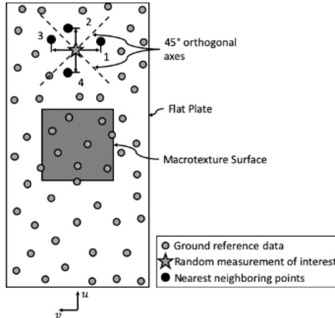
Figure 63. Illustration of four quadrants oriented with respect to the path coordinate system and identification of the nearest neighboring point in each respective quadrant for an example measurement of the flat plate.
