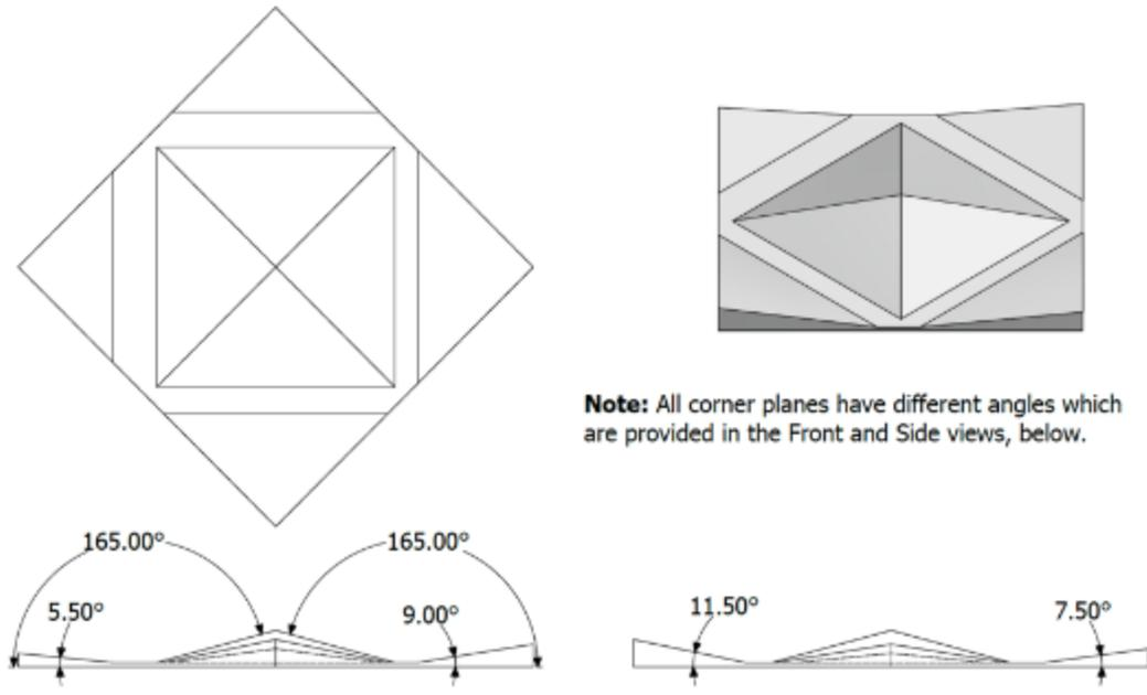
Figure 70. Dimensions of the angled surfaces associated with the reference object used for the navigation drift assessment during the second equipment rodeo.
