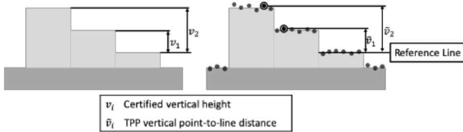
Figure 37. Example vertical point-to-line distance between two horizontal surfaces on a gauge block to provide an estimation of the TPP reported vertical height between gauge block surfaces.
