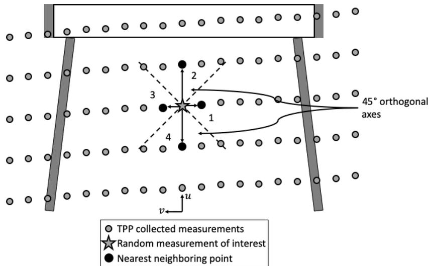
Figure 46. Illustration of four quadrants oriented with respect to the path coordinate system and identification of the nearest neighboring point in each respective quadrant.
