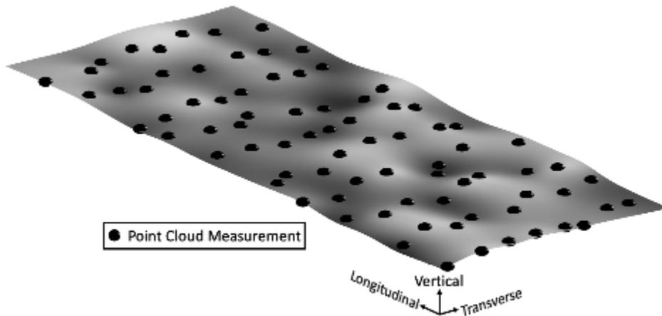
Figure 4. Generalized representation of point cloud measurements from a TPP for a road surface.
