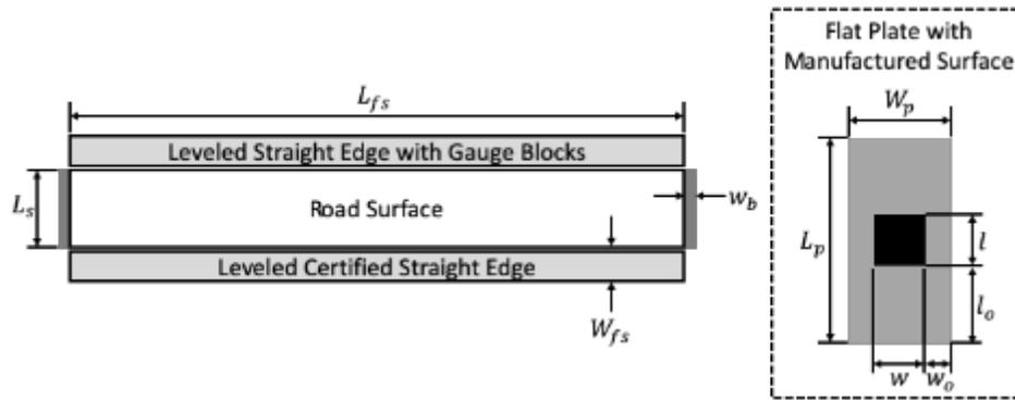
Figure 57. General layout of the test section with the bounding straight edges and manufactured surface off to the side of the road surface of interest.
