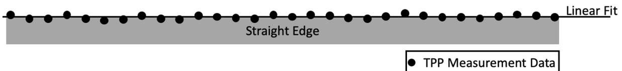
Figure 11. Linear fit to measurement points for determining straightness.
