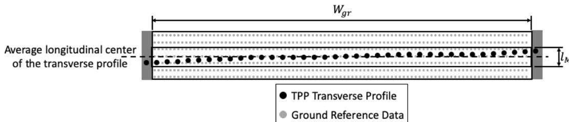
Figure 54. Identification of the ground reference data points for calculation of reference cross-slope and rut-depth.
