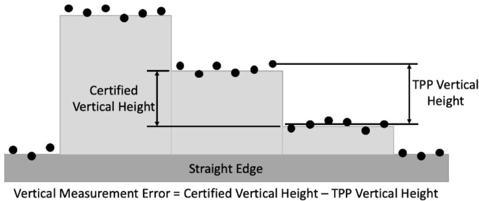
Figure 10. Example vertical measurement error for TPP measurements of a certified gauge block resting on a straight edge.
