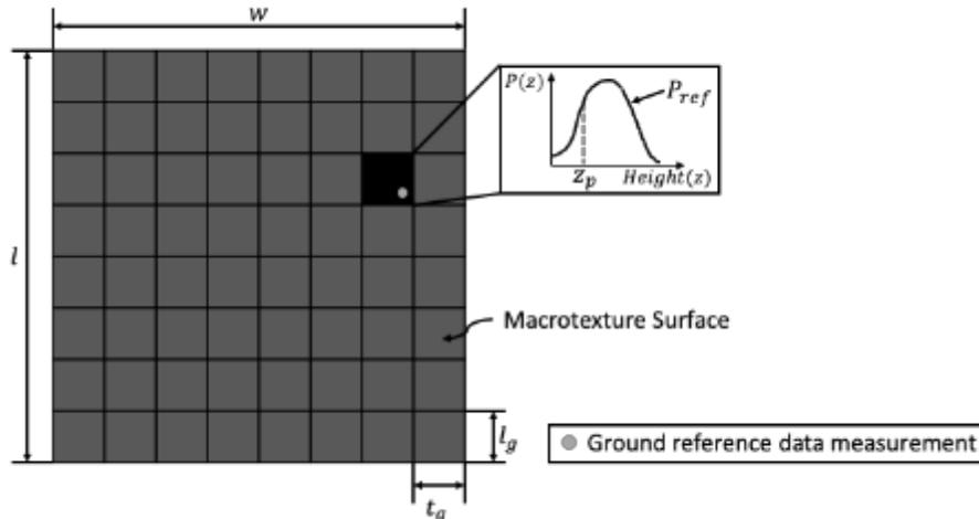
Figure 64. Gridding to determine the vertical accuracy and precision of ground reference data on a manufactured surface.
