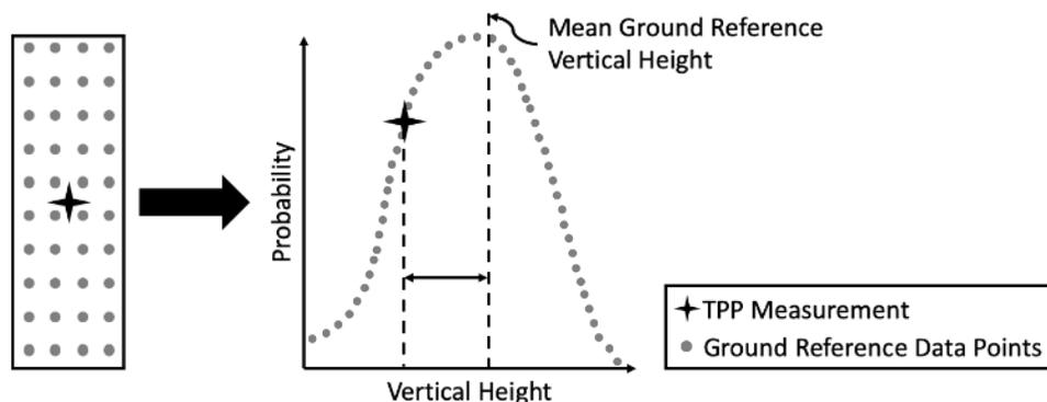
Figure 18. Evaluation of TPP measurement to ground reference distribution.
