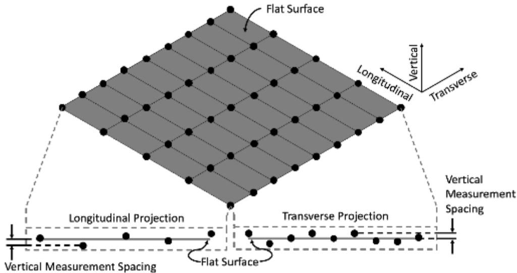
Figure 8. Illustration of vertical measurement spacing for a set of TPP measurements which lie on a flat surface.
