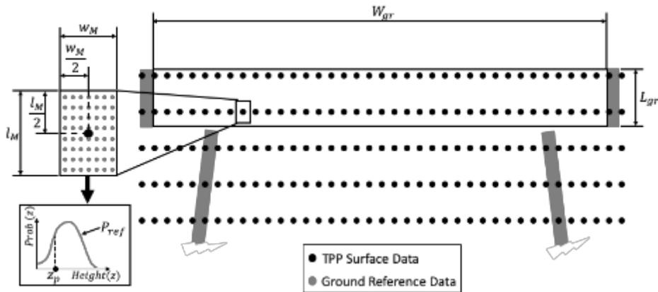
Figure 52. Ground reference rectangular region of interest to determine gridded data vertical error.
