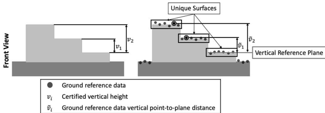
Figure 60. Identification of unique surfaces of a gauge block corresponding to vertical error measurement in the ground reference data point cloud, and example vertical point-to-plane distances for each unique surface set.
