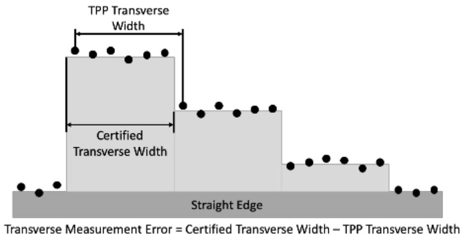
Figure 9. Example transverse measurement error for TPP measurements of a certified gauge block resting on a straight edge.
