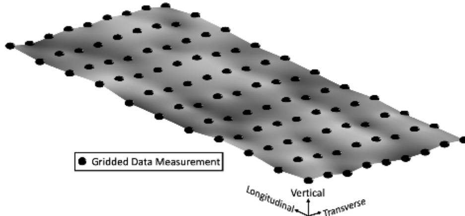
Figure 5. Generalized representation of gridded data measurements from a TPP for a road surface.
