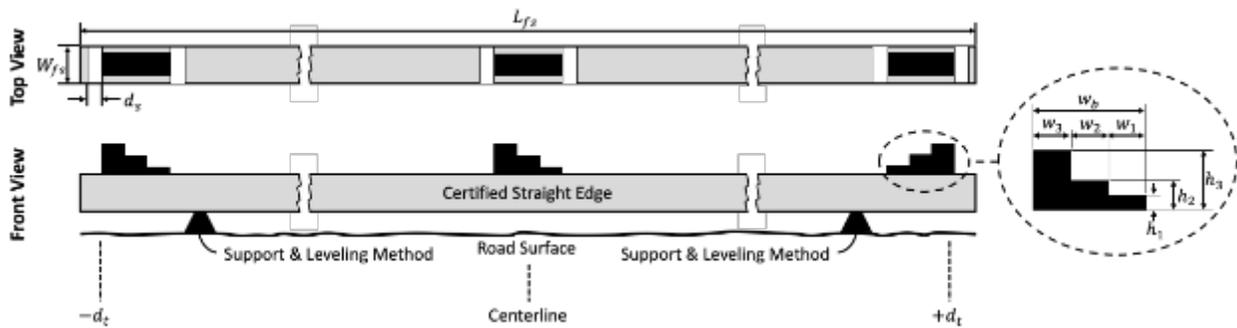
Figure 32. Layout of the stair-stepped gauge blocks at the center, left, and right side of the straight edge.
