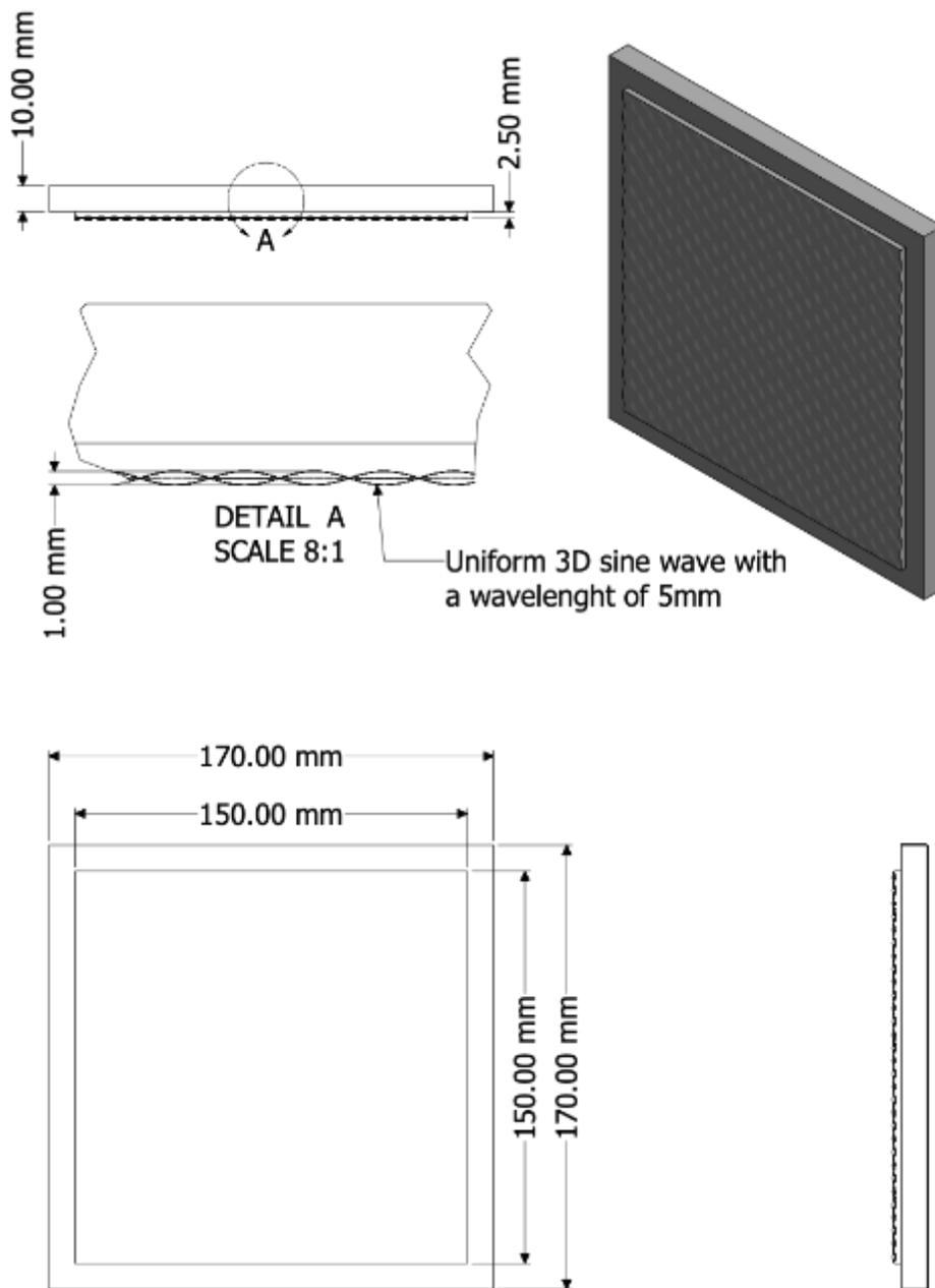
Figure 71. Dimensioned drawing of the macrotexture surface used during the assessment of ground reference data.
