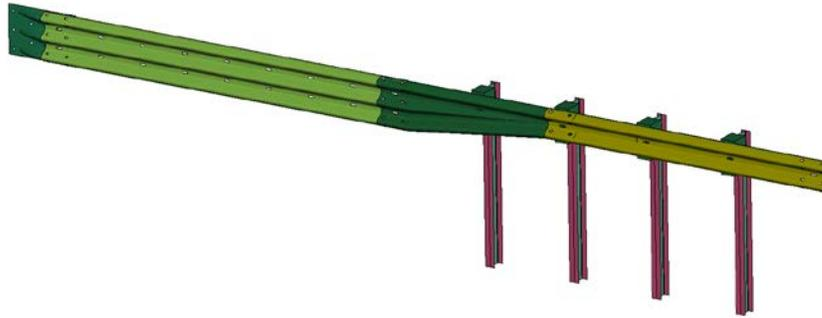
Figure 2. Model of MGS Transition
