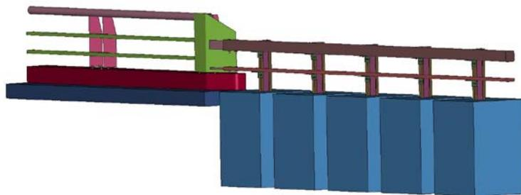
*Figure 1. Model of Box Beam Transition to C2P Bridge Rail*
