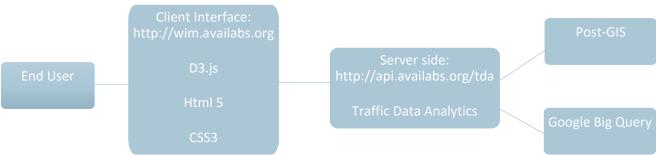
Figure 4 Web-Based Analysis Tool Software Architecture with Software Names
