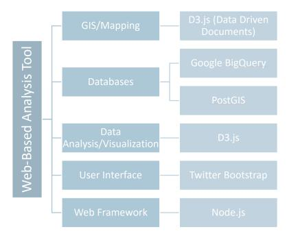
Figure 3 Web-Based Analysis Tool, Software by Function
