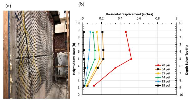
Fig. 8 (a) photograph of MSE wall panel deflection at failure, and (b) measured horizontal deflection of the wall versus height above the base of the wall for selected surcharge pressures.
