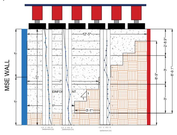
Fig. 9 Cross-section showing settlement vs. depth profiles from vertical Sondex pipes.
