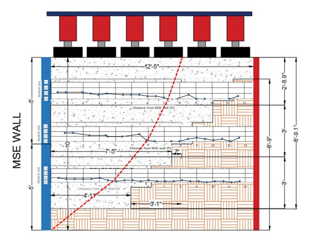
Fig. 10 Cross-section showing elongation vs. distance plots from horizontal Sondex pipes.
