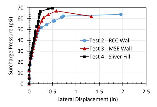
Fig. 6. Comparison of applied surcharge pressure vs. lateral displacement for LCC backfill tests with a reinforced concrete cantilever wall (RCC), MSE wall, and a MSE wall with a sliver fill.
