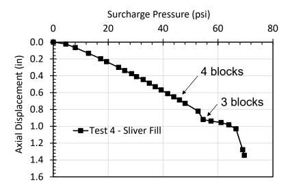
Fig. 3. Applied surcharge pressure versus axial displacement for the sliver fill test.
