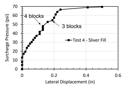
Fig. 5. Applied surcharge pressure vs. lateral displacement at the MSE wall for the sliver fill test.
