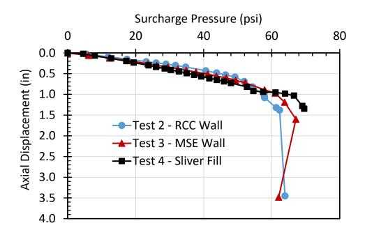
Fig. 4 Comparison of applied surcharge pressure vs. axial displacement for LCC backfill tests with a reinforced concrete cantilever wall (RCC), MSE wall, and a MSE wall with a sliver fill.
