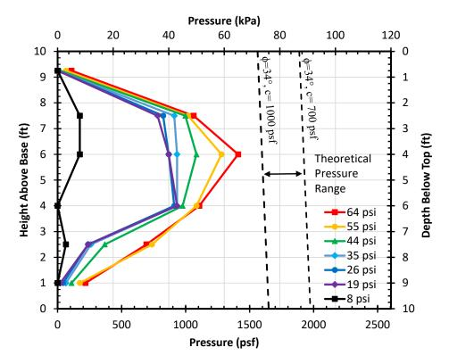
Fig. 7. Horizontal pressure on the MSE wall vs. depth curves for selected applied surcharge pressure values near the wall during the MSE sliver fill test from Geokon pressure plates.
