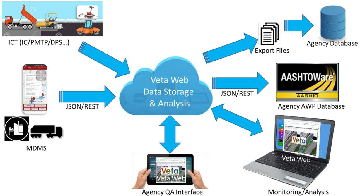
The MDMS data will be stored on the server with data security and integrity. Veta Web will be used for managing users, data-access permissions, and MDMS projects. While Veta Web will interact with the server, the time-intensive calculations will be performed on the server. This includes filtering, analyzing, reporting, and map creation similar to those in the current Veta desktop version. Specifically, the following features:
