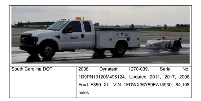
Additionally, two Continuous Friction Measuring Equipment (CFME) Devices were part of the event this year.
