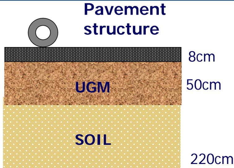
Loading : 65 kN load (single or dual wheel)
