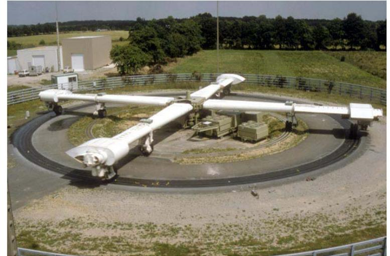
“FABAC” Machines : mobile machines – simulation of full wheel loading on small length (2m)
