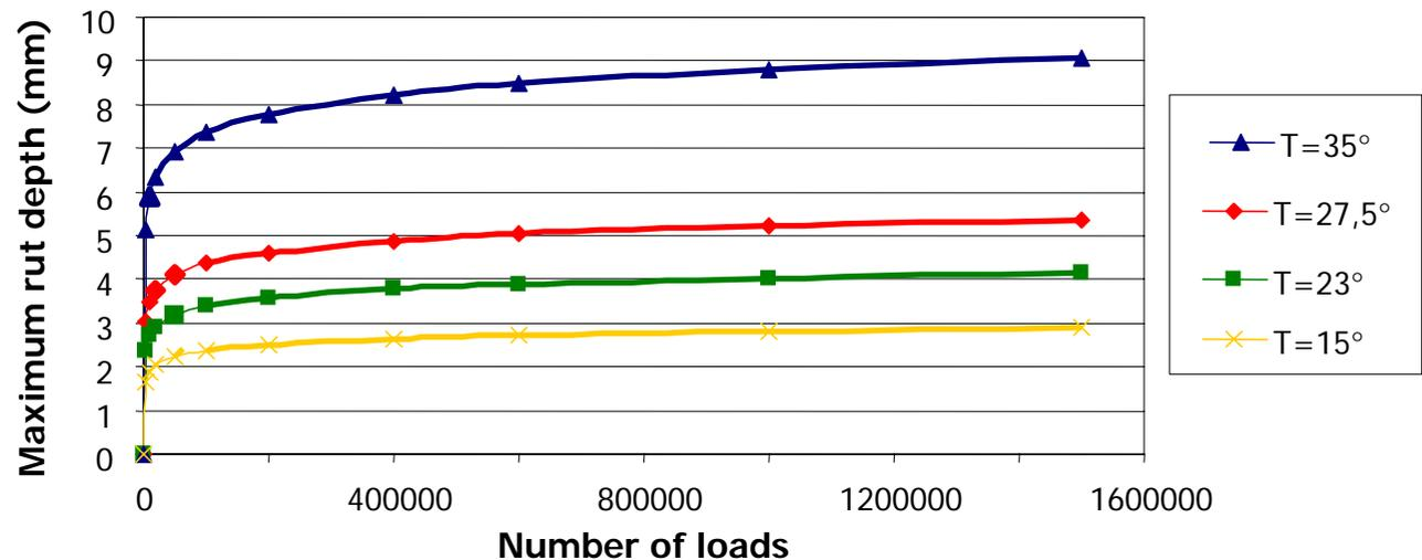
Rut profiles for different Temperatures (8.5 to 42.5°C)
