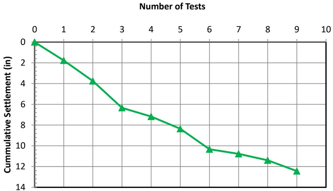
Figure 65 Cumulative Settlement for all Tests During PVD-1
