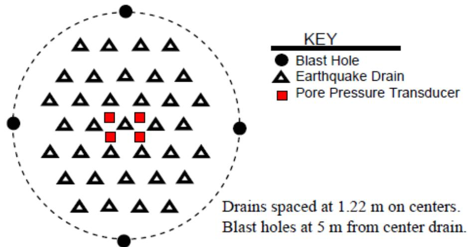
**Figure 5 Layout of EQ Drains, Blast Holes and Pore Pressure Transducers to Monitor Effectiveness of Drains for Liquefaction Remediation.**
