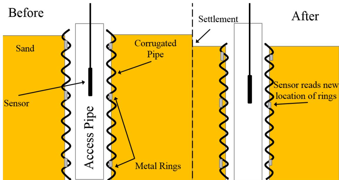
**Figure 27 Profile View of Sondex Settlement Profilometer**
