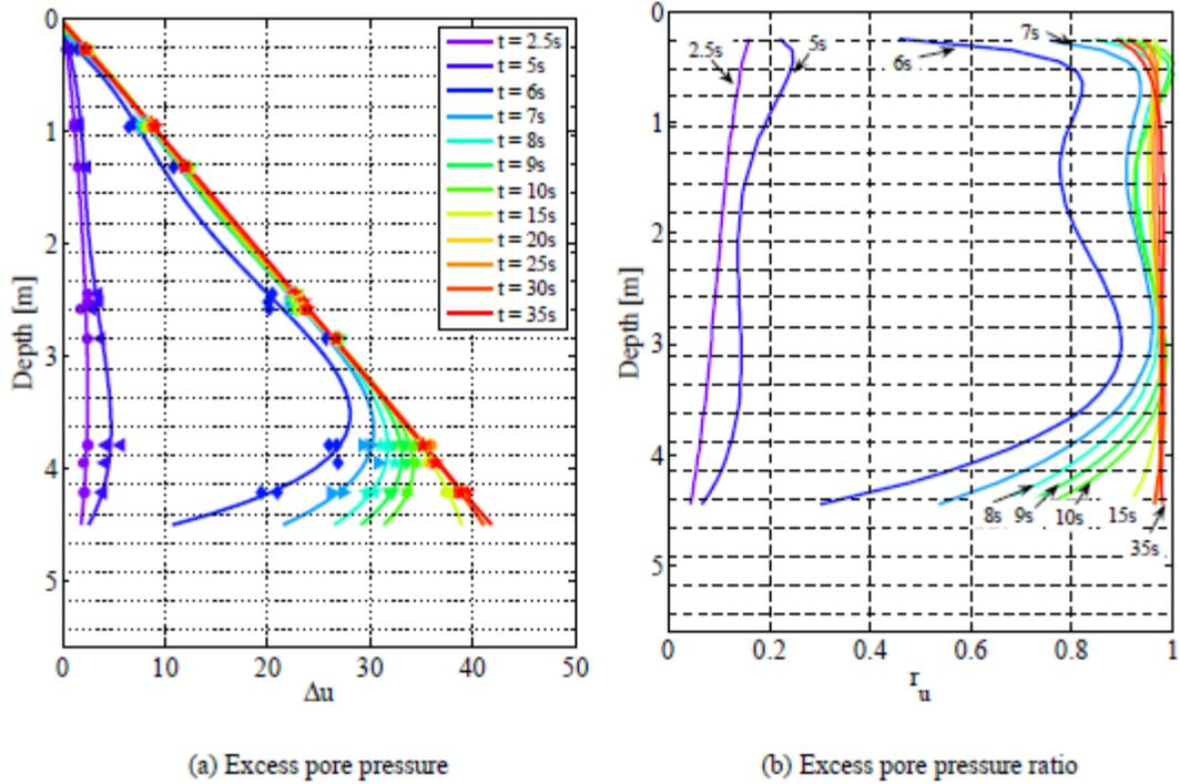
Figure 18 Excess Pore Pressure Profiles for LG0 (Bethapudi 2008).
