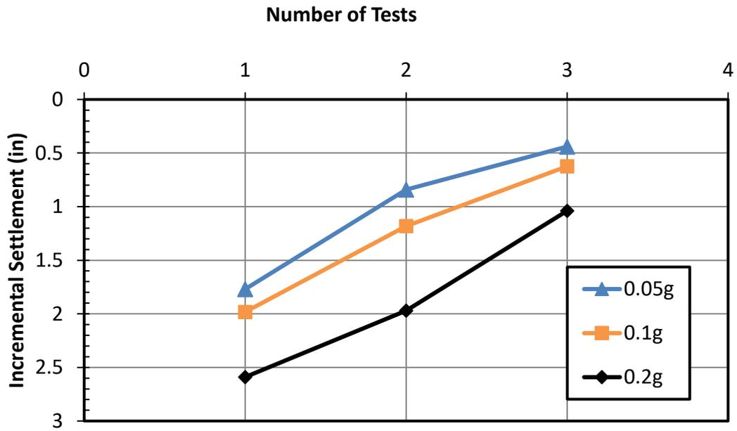
**Figure 67 Incremental Settlement at a Given Peak Acceleration**
