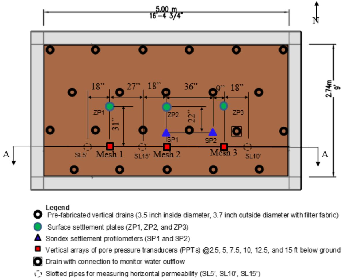
Figure 73 Plan View of Sensors for PVD-2
