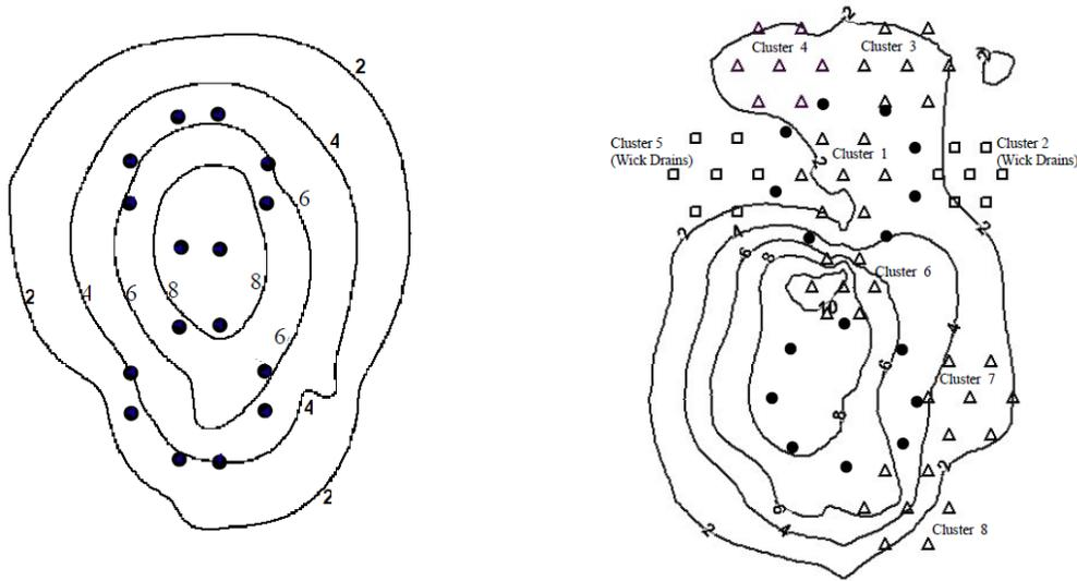
**Figure 4 Contours of Measured Settlement (in cm) for (A) Untreated Site and (B) Site Treated with Clusters of EQ Drains After Detonation of 16 Explosive Charges Around Two 4.3 M Diameter Rings. Rollins et al, (2003).**
