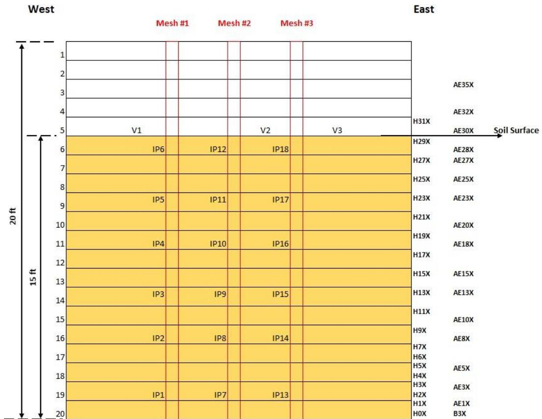
**Figure 30 Profile View of Sensors Installed for PVD-1**
