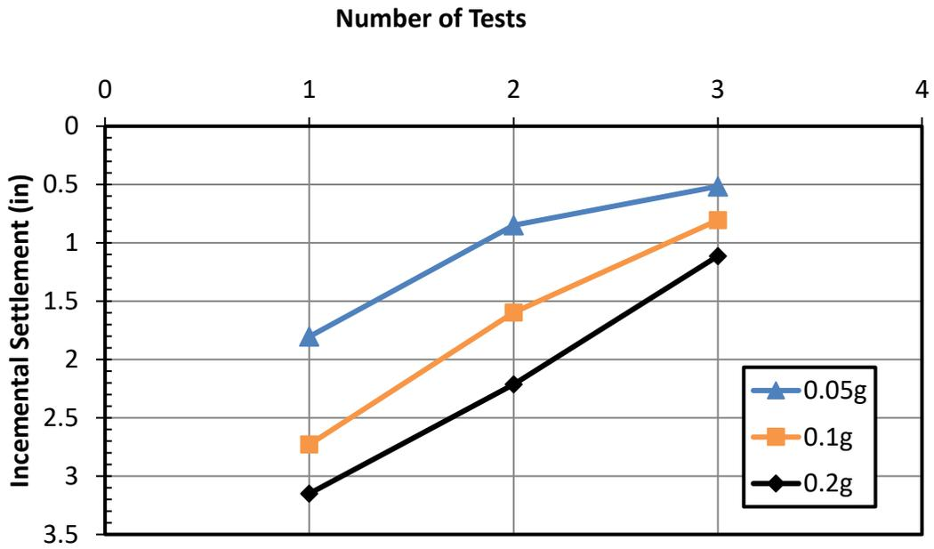
Figure 108 Incremental Settlement at a Given Peak Acceleration
