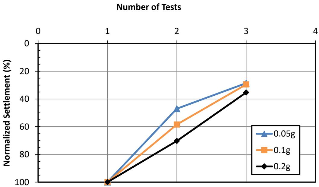
Figure 109 Settlement of Sand with Number of Tests at a Given Acceleration Level After Normalization by Settlement for the First Round
