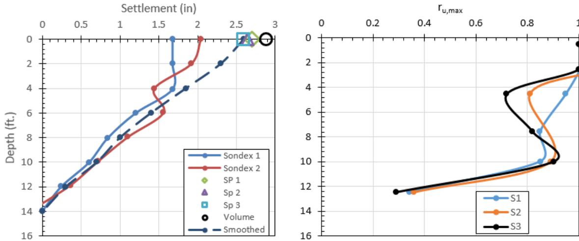
**Figure 52 Profiles of Liquefaction Induced Settlement and Maximum Excess Pore Pressure Ratio ( $r_{u,max}$ ) for Round 1 Test with  $a_{max}=0.20$  g.**
