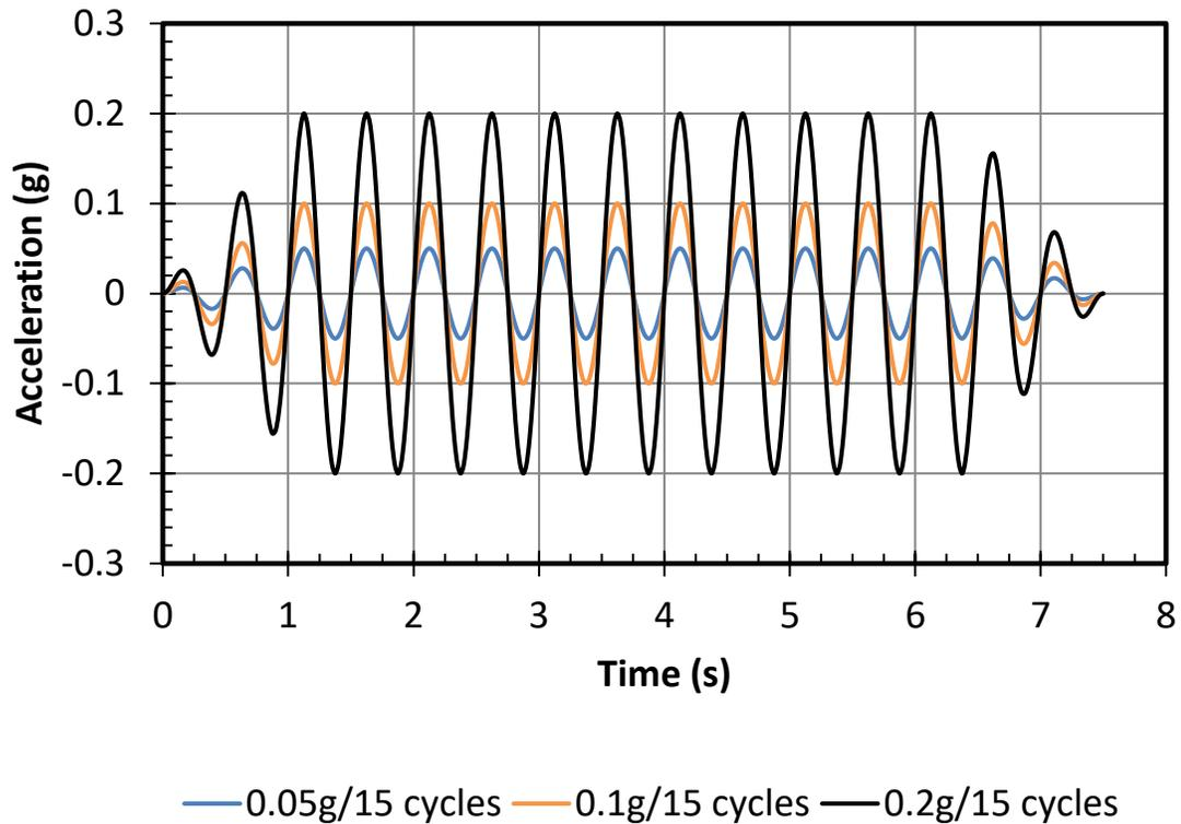
**Figure 79 Input Motions for Each Set of Three Tests**
