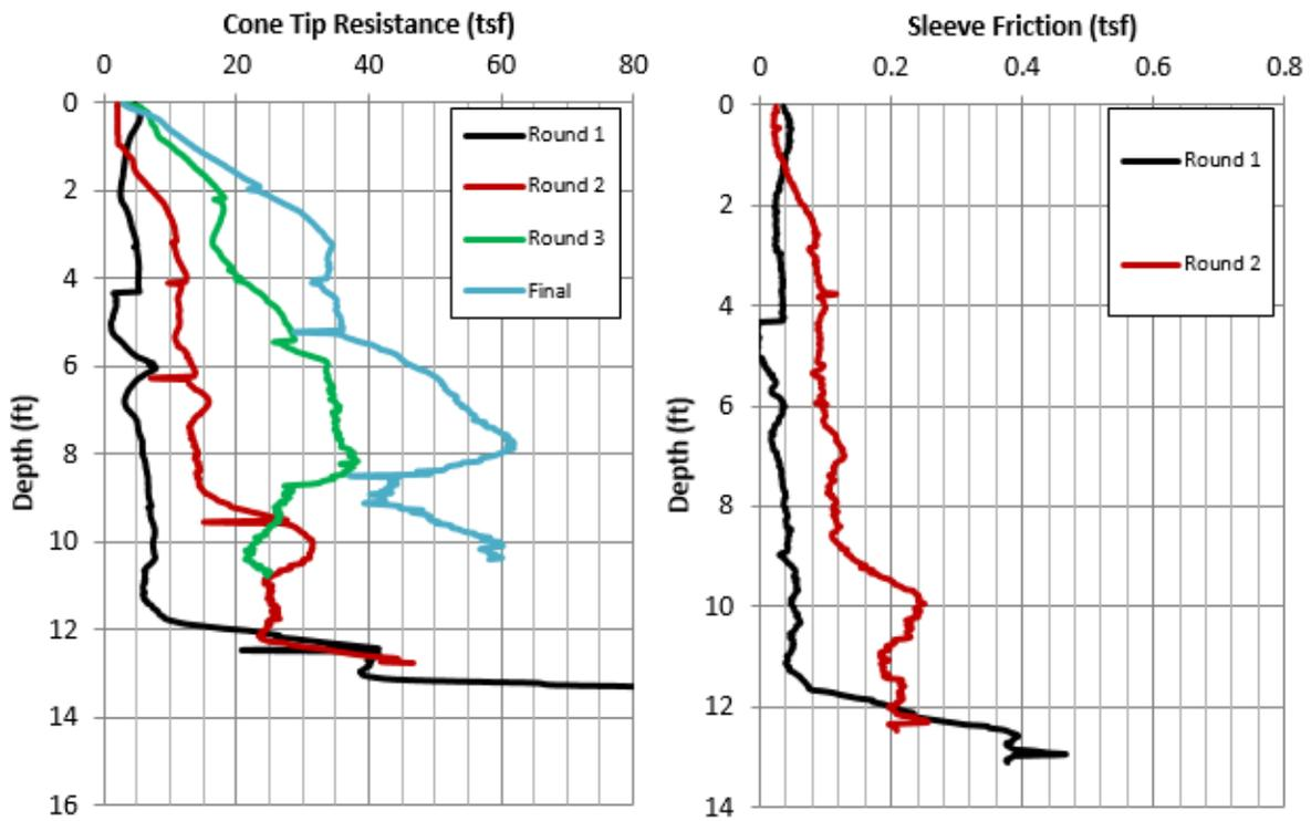
Figure 35 CPT Cone Tip Resistance Values for PVD-1.
