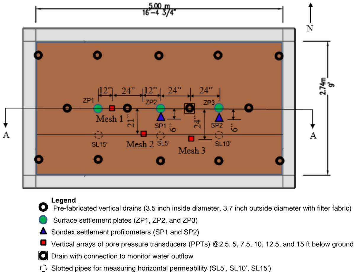
**Figure 29 Plan View of Sensors for PVD-1**
