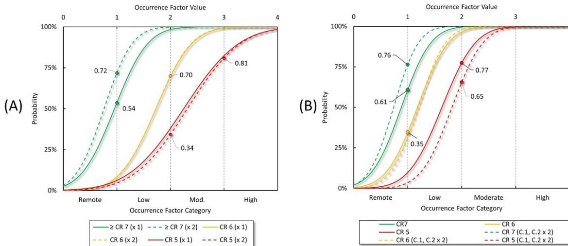
Figure 1. Results from back-casting (A) and Monte Carlo simulations (B) for bridge deck components.
