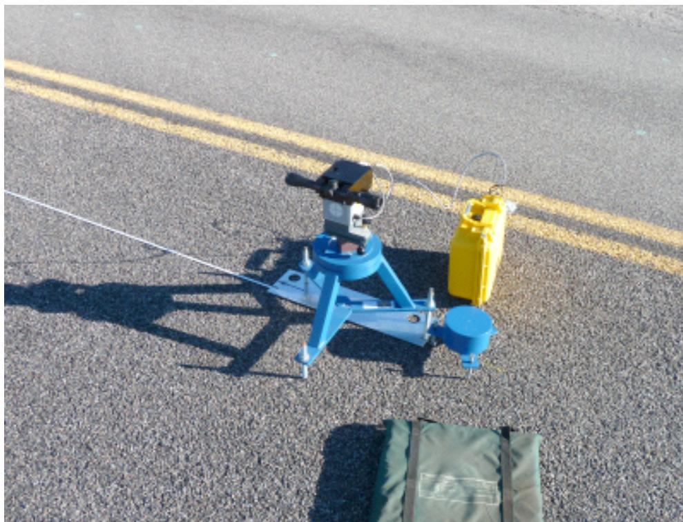
**Figure B–4. Benchmark Profiler reference laser stand and guide tape, 2010.**
