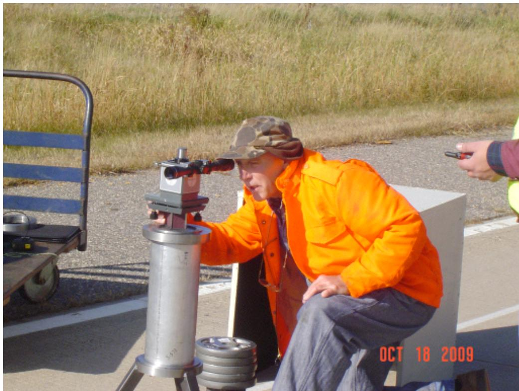
**Figure B–3. Benchmark Profiler reference laser set-up, 2009.**
