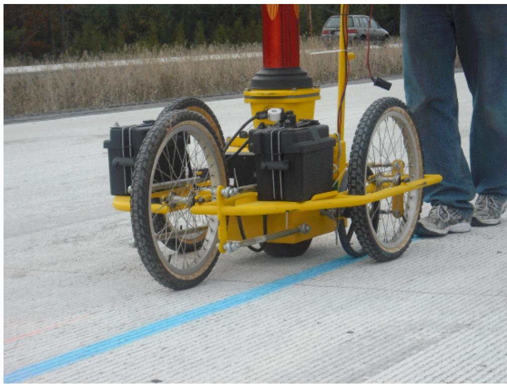
**Figure B–11. APR Auto Rod and Level, close-up, 2009.**
