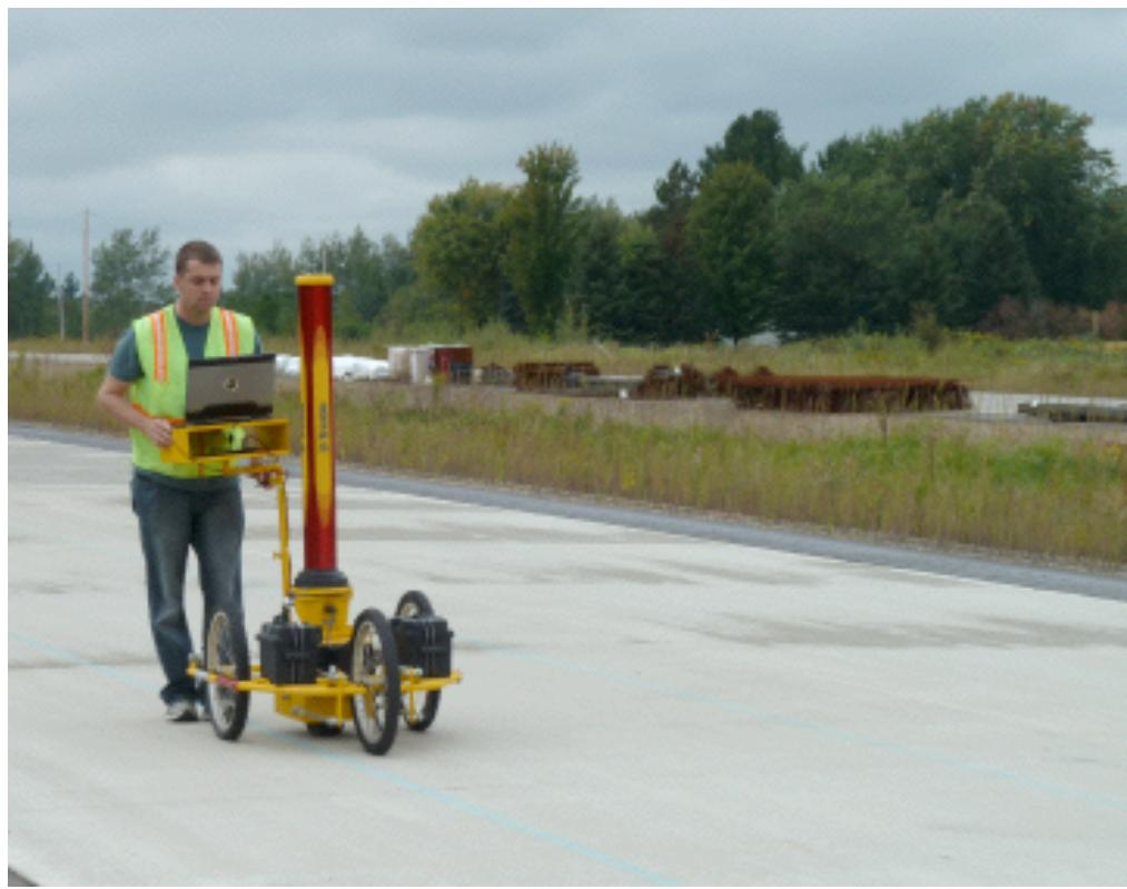
**Figure B–12. APR Auto Rod and Level, front view, 2010.**
