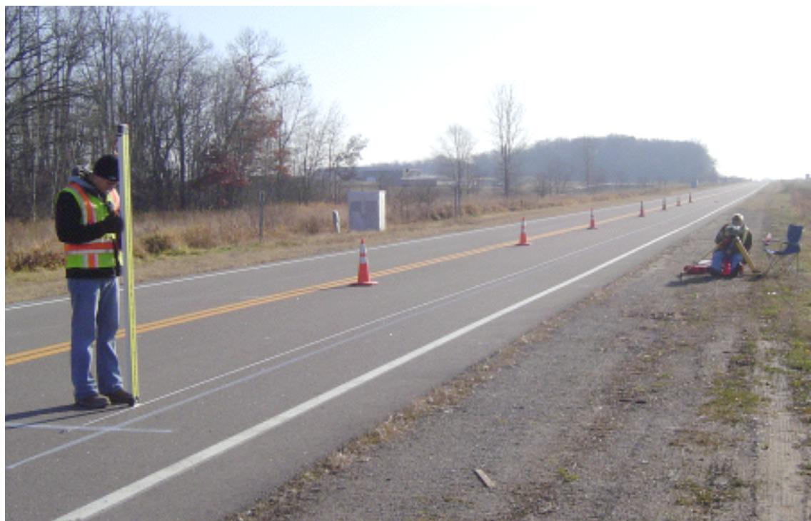
**Figure B–8. Surveyor's rod and level, 2009.**
