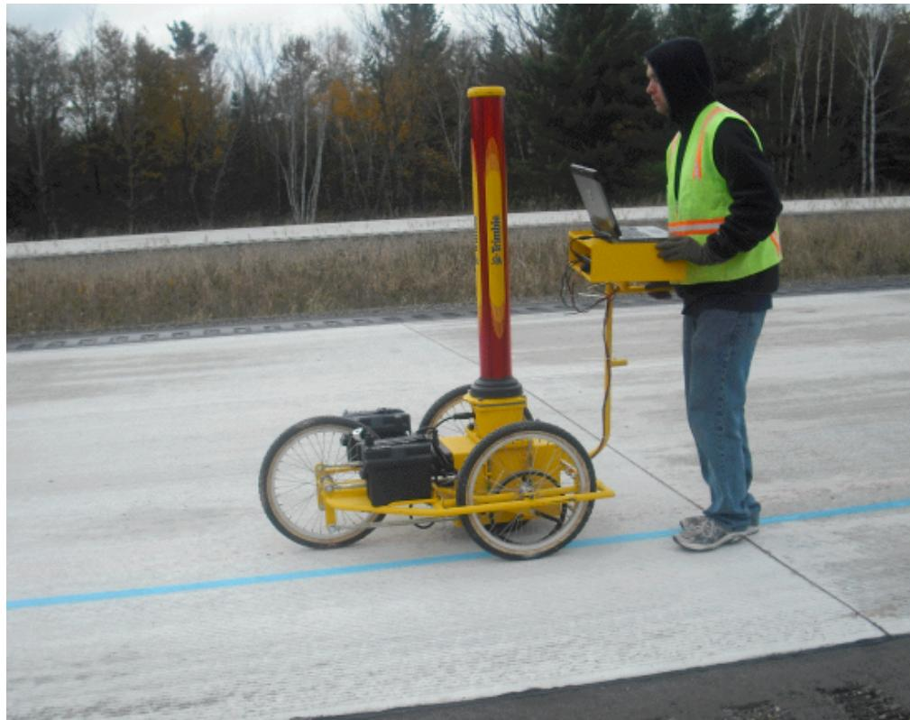
**Figure B–10. APR Auto Rod and Level, side view, 2009.**
