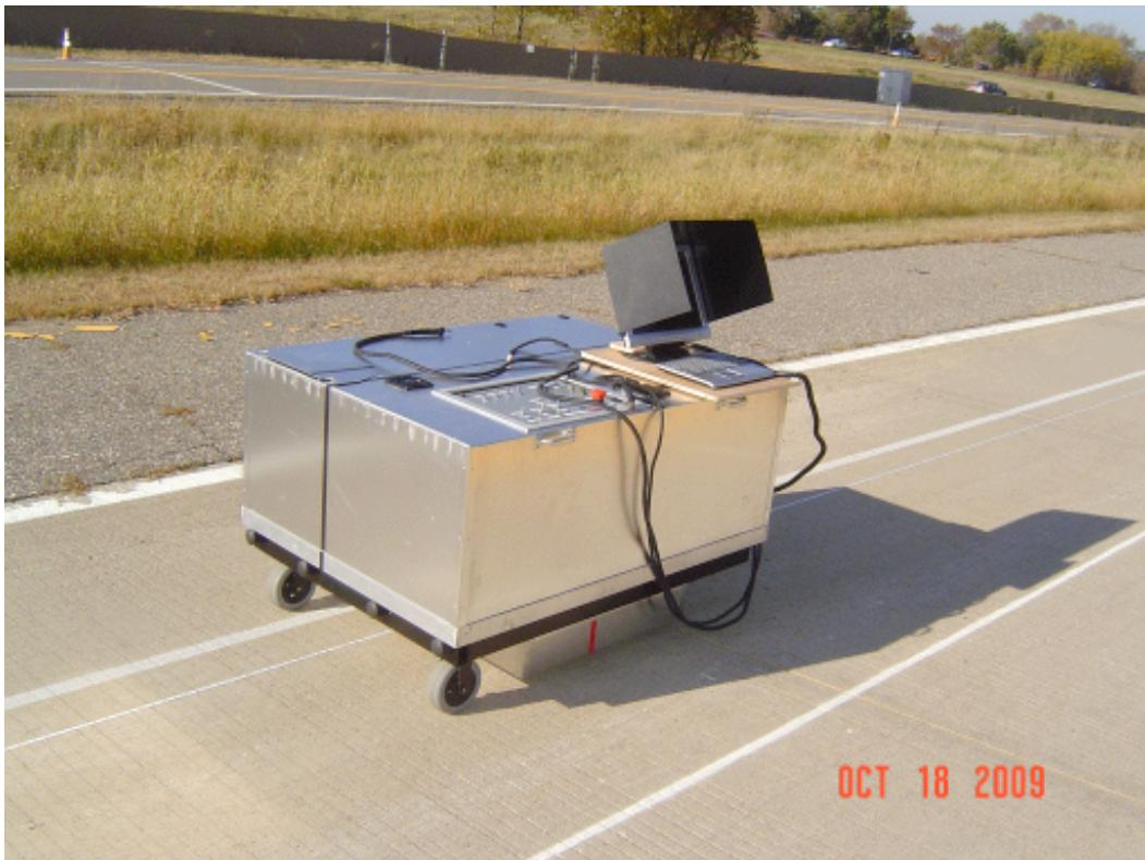
**Figure B–1. Benchmark Profiler cart, left front view, 2009.**
