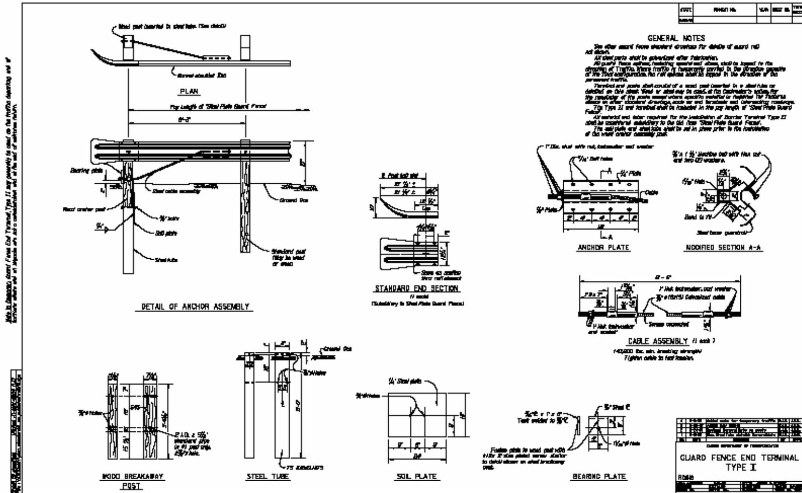
Figure 1. Type II Guard Fence End Terminal Standard Drawing
