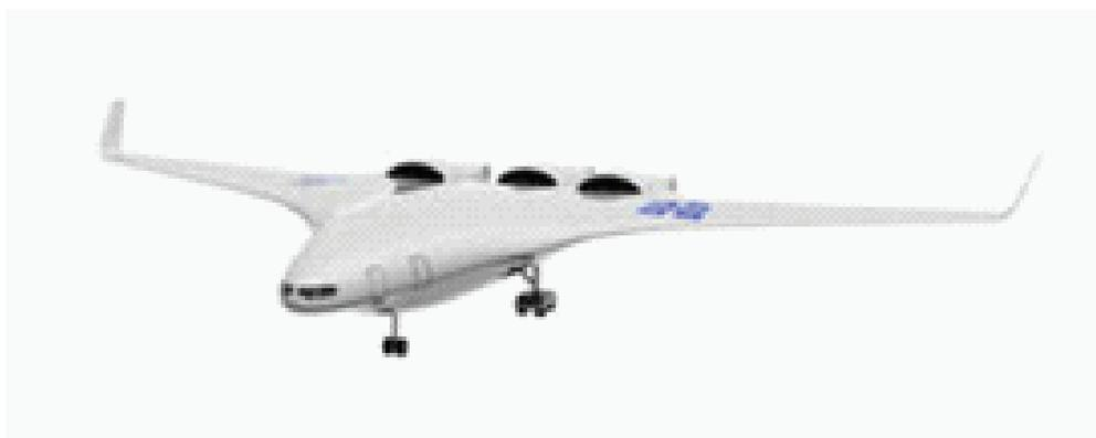
FIGURE 5-12 SAX-40 silent aircraft. Source: SBAC (2009). Copyright Silent Aircraft Initiative.
