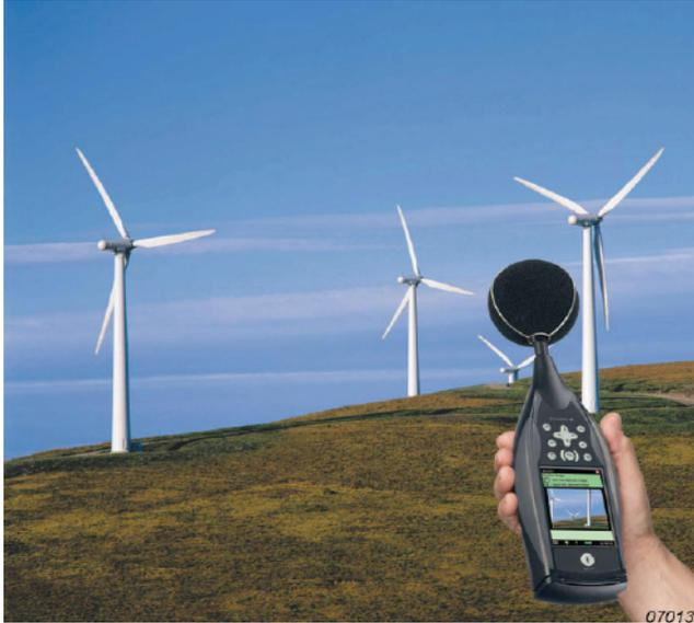
FIGURE E-2 Type 2270 meter in use. Copyright © Brüel & Kjær.
