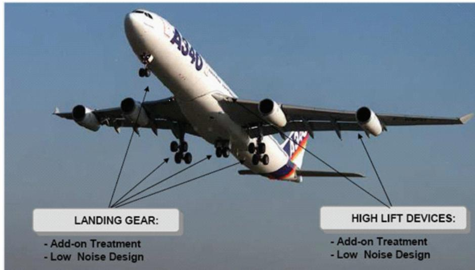
FIGURE 5-10 Aircraft noise reduction technologies. Source: SBAC (2009).
