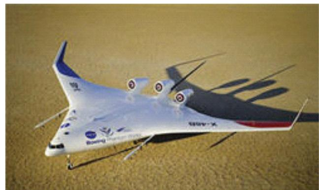
FIGURE 5-15 Hybrid wing/body aircraft with vertical tails on either side of the engines to shield jet noise. Source: NASA (2002).
