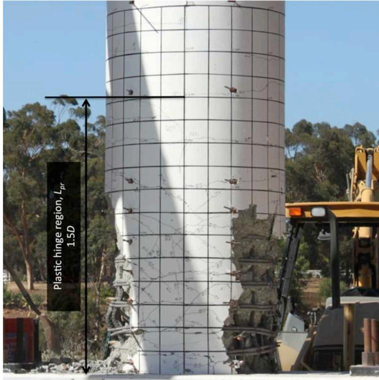
**Figure 9.5 South face of the column post-test.**
