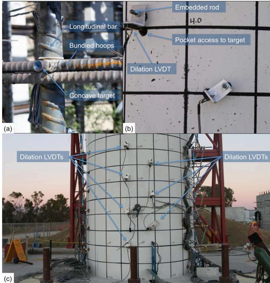
**Figure 7.4 Dilation LVDT installation (a) target welded to a transverse hoop, (b) LVDT assembly, and locations on the West face.**
