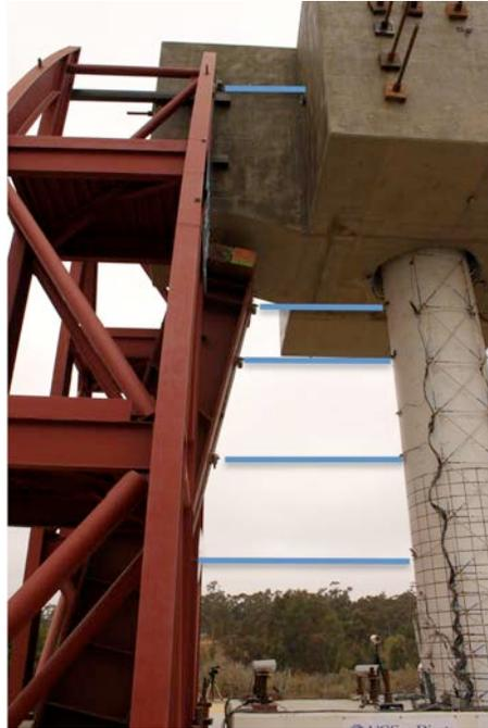
**Figure 7.5 Horizontal spring potentiometer locations.**
