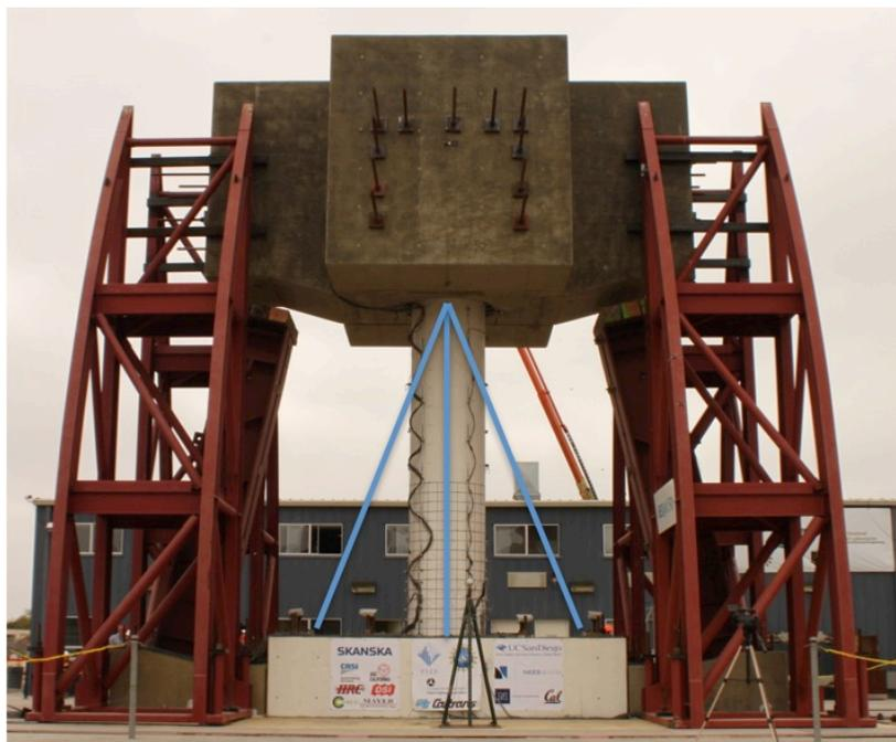
**Figure 7.6 Inclined spring potentiometer locations.**
