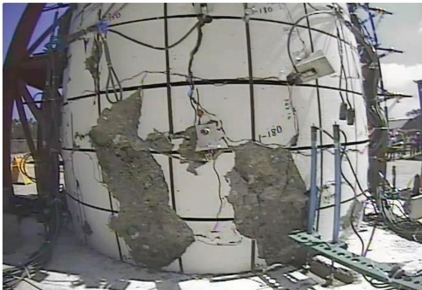
**Figure 8.15 Column base West face after test EQ3.**
