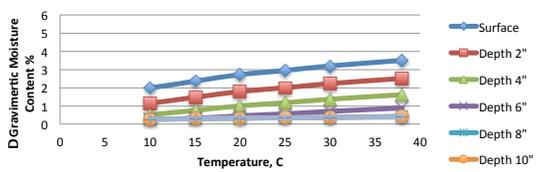
DMC in depth Vs. Temperature: fine Sand 24 hrs after placement
