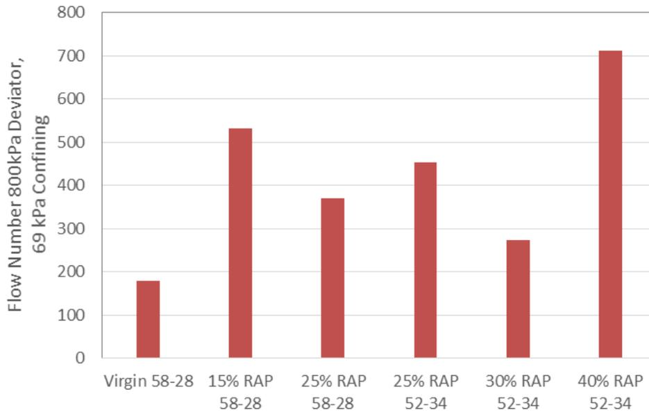
Figure 3.42 Average Flow Number for PMPC Specimens at 69 kPa Confining Pressure and 800 kPa Deviator Stress
