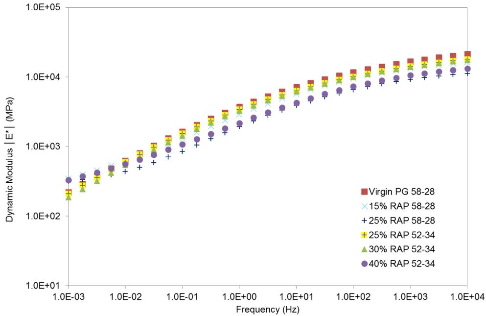
Figure 3.23 Average Dynamic Modulus Master Curves at 21°C for PMLC Specimens
