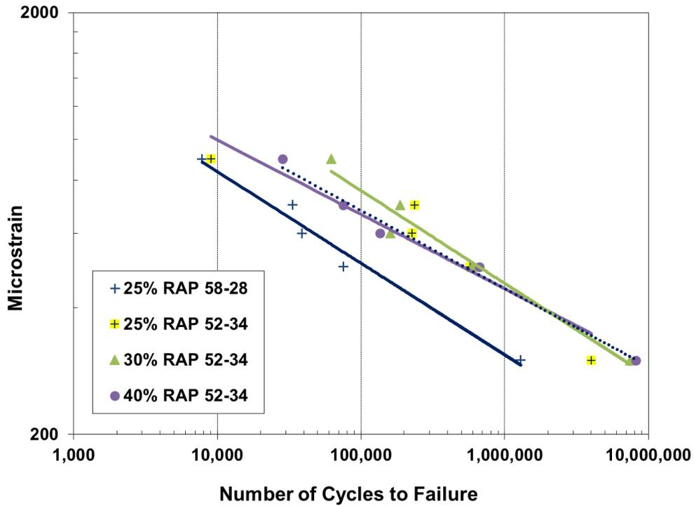
Figure 3.37 Flexural Beam Fatigue Results for NH Mixtures
