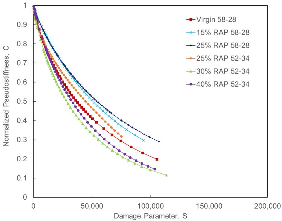
Figure 3.31 Damage Characteristic Curves for PMPC Specimens
