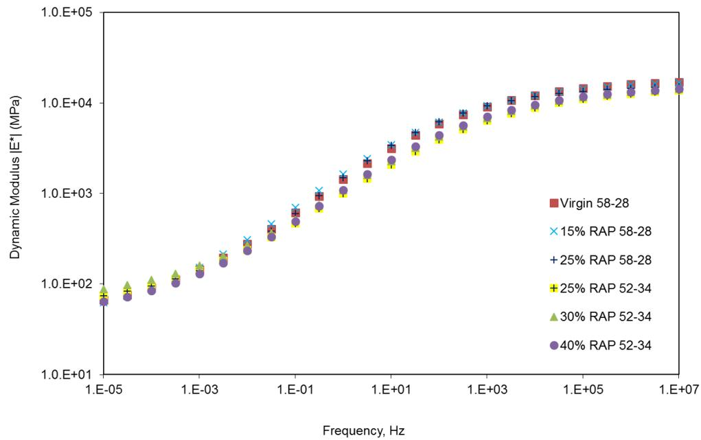
Figure 3.13 Average FHWA PMPC Dynamic Modulus Master Curves at 21°C for All Production Days
