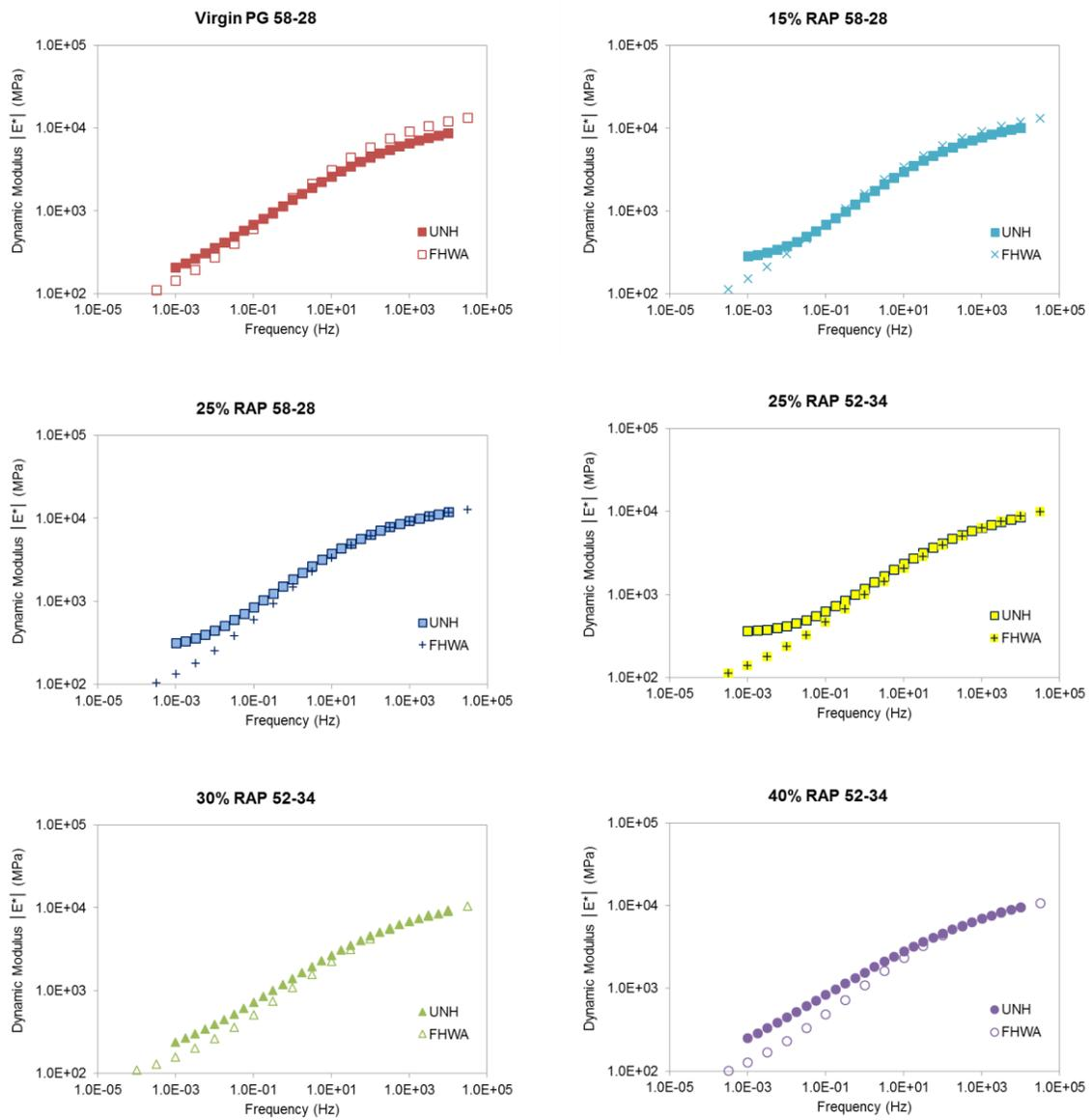
Figure 3.27 Comparison between UNH and FHWA PMPC Dynamic Modulus Master Curves at 21°C
