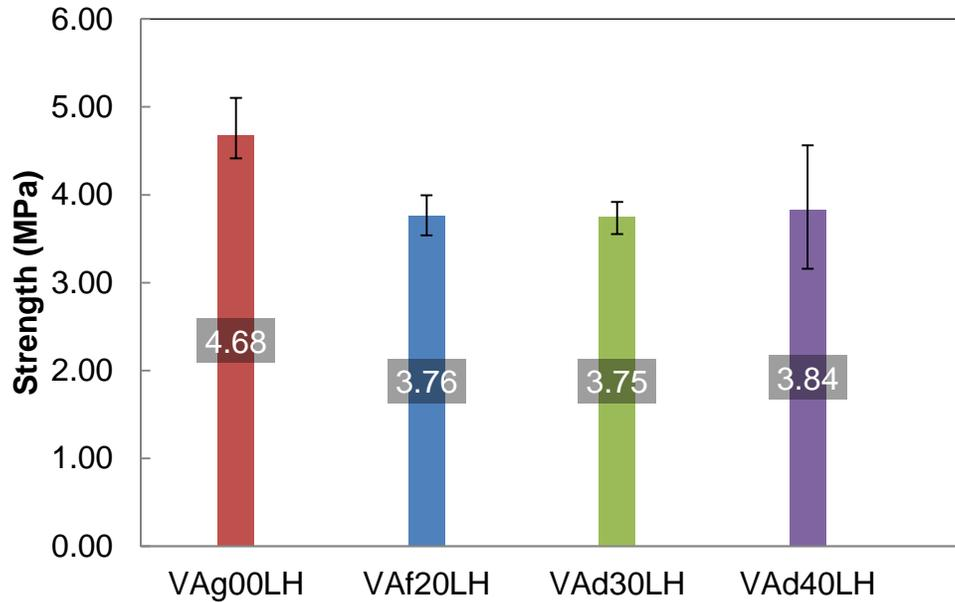
Figure 4.10 Low temperature strength results for VA PMLC Specimens
