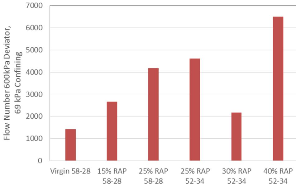
Figure 3.40 Average Flow Number for PMPC Specimens at 69 kPa Confining Pressure and 600 kPa Deviator Stress
