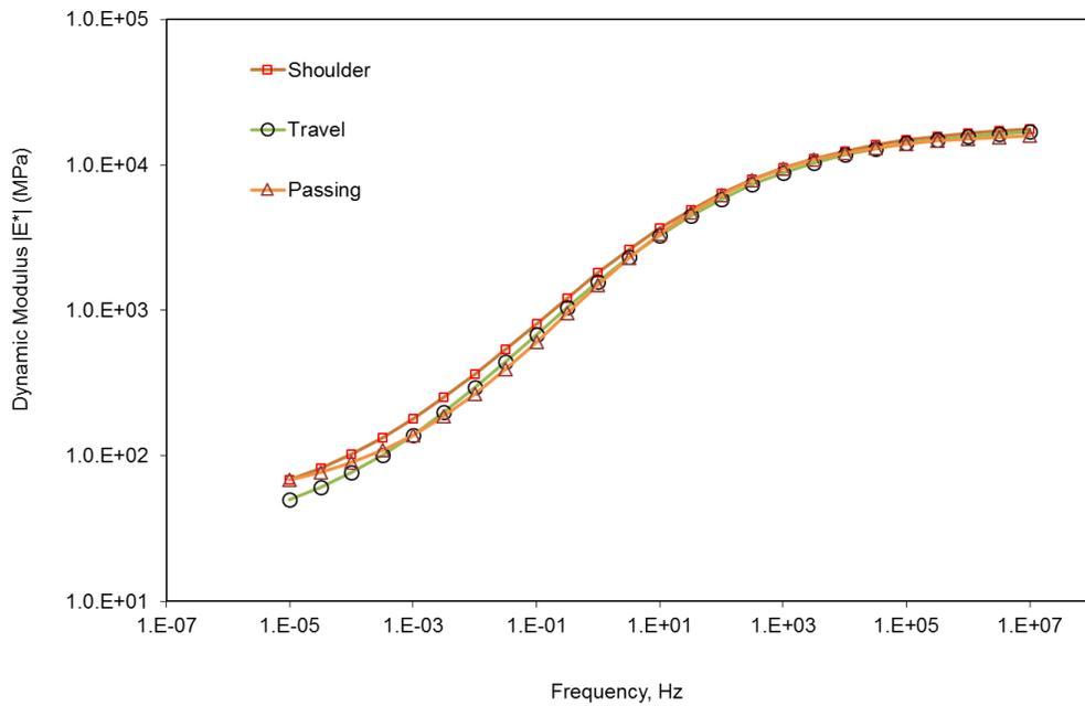
Figure 3.16 15% RAP PG 58-28 Average Dynamic Modulus Curves at 21°C for all PMPC Production Days
