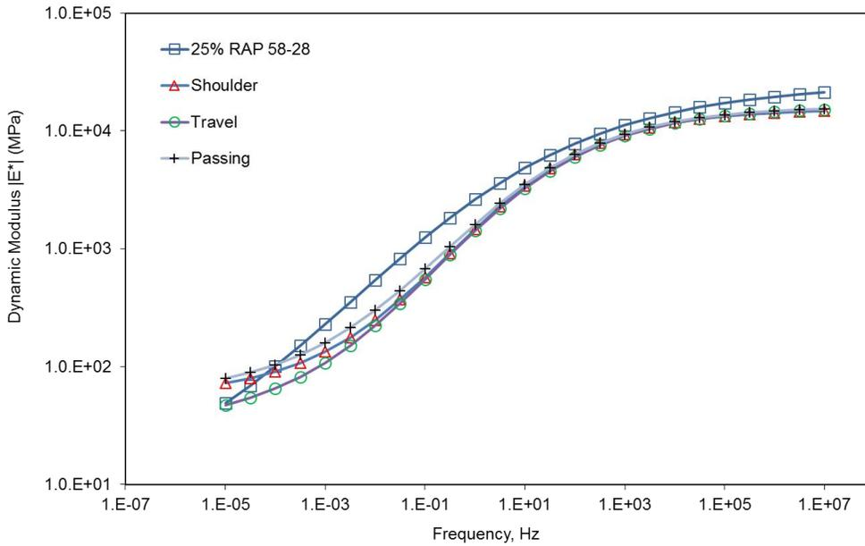
Figure 3.17 25% RAP PG 58-28 Average Dynamic Modulus Curves at 21°C for LMLC and all PMPC Production Days
