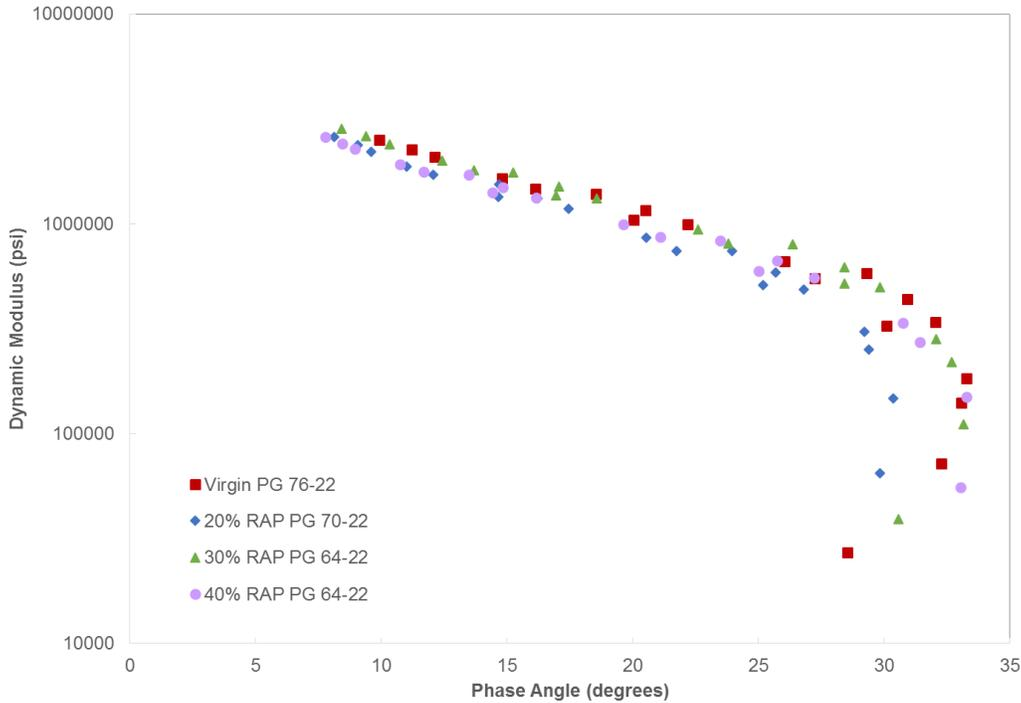
Figure 4.2 Black Space Curves for VA PMLC Specimens
