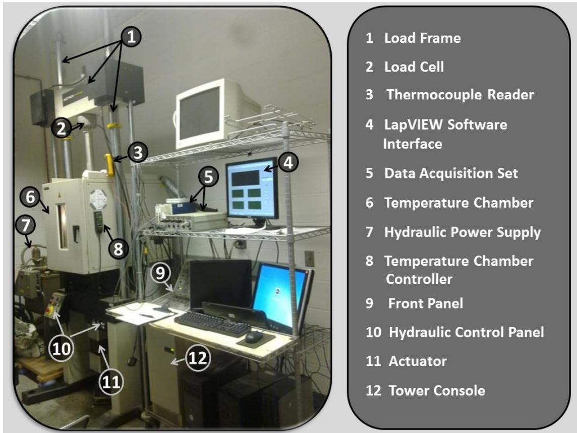
Figure 2.6 A closed-loop servo-hydraulic system manufactured by Instron Inc.
