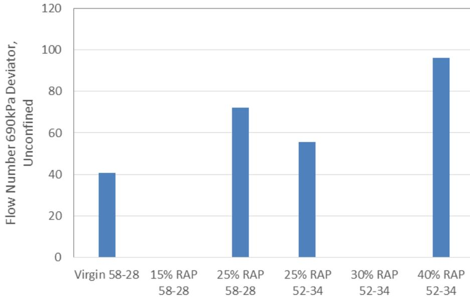
Figure 3.39 Average Flow Number for LMLC Specimens Unconfined and 690 kPa Deviator Stress
