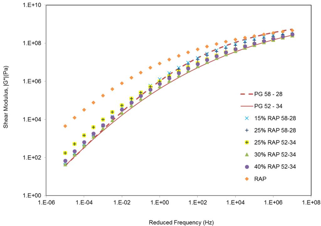
Figure 3.9 Shear Modulus Master Curves at 21°C for Virgin and Extracted and Recovered Binders
