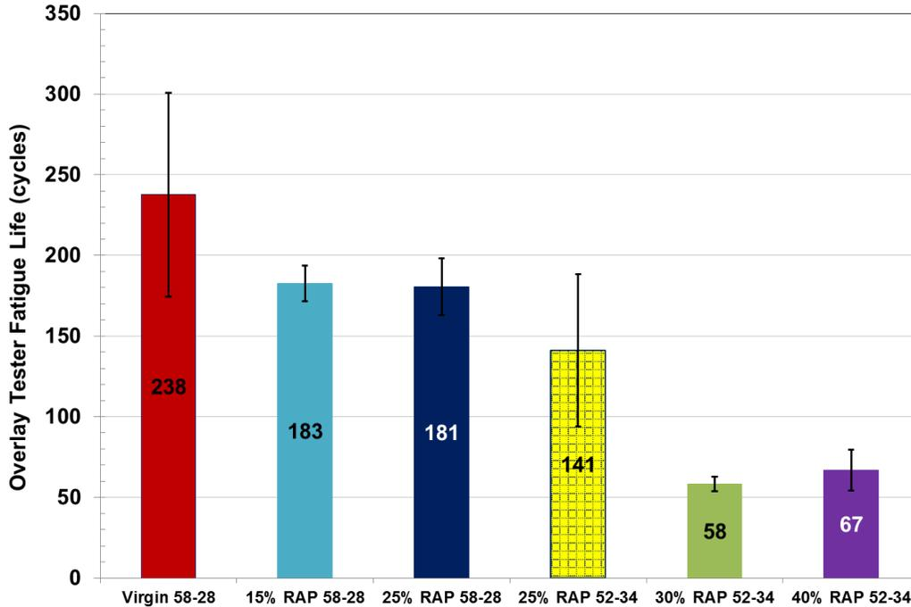
Figure 3.38 Overlay Tester Results for NH Mixtures
