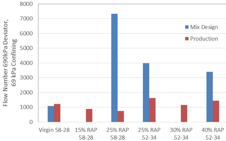
Figure 3.41 Average Flow Number for LMLC and PMPC Specimens at 69 kPa Confining Pressure and 690 kPa Deviator Stress
