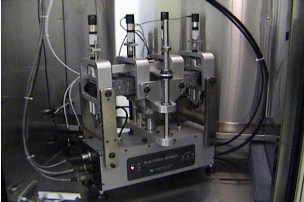
Figure 2.4 Flexural beam fatigue test apparatus
