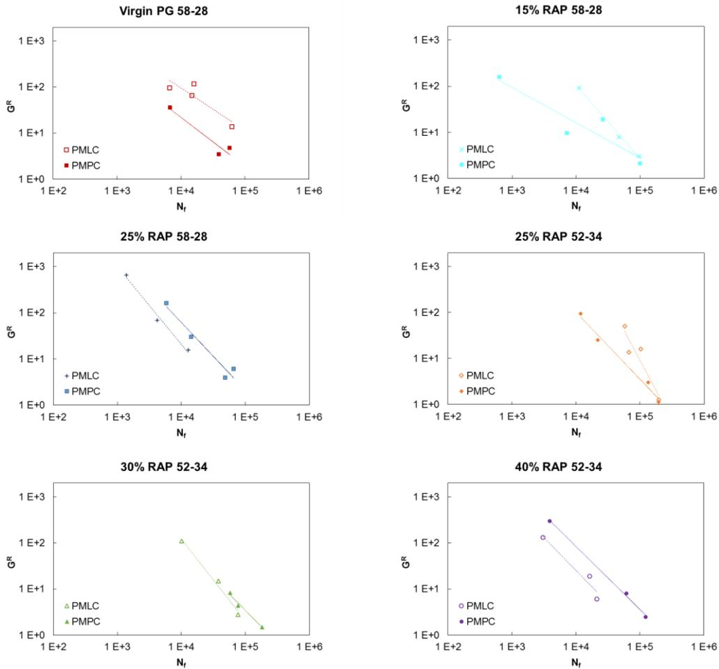
Figure 3.36 Comparison of PMLC and PMPC  $G^R$  versus number of cycles to failure curves for each mixture
