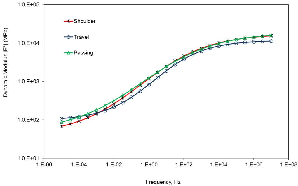
Figure 3.19 30% RAP PG 52-34 Average Dynamic Modulus Curves at 21°C for all PMPC Production Days
