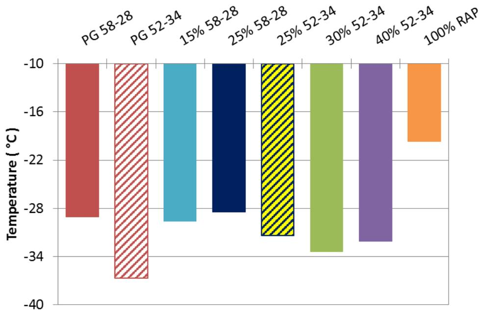
Figure 3.7 Continuous Low Temperature Grade for Virgin and Extracted and Recovered Binders
