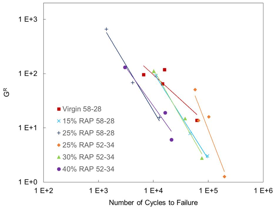
Figure 3.34  $G^R$  versus Number of Cycles to Failure for PMLC Specimens
