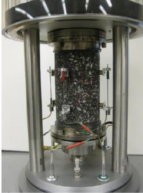
Figure 2.1 LVDT mounting and spacing for SVECD Fatigue
