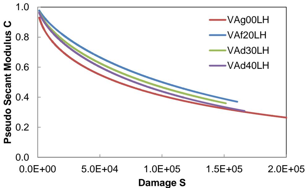
Figure 4.3 Characteristic curve C vs. S - all VA mixtures
