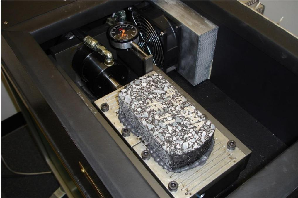
Figure 2.5 Overlay tester with a mounted test specimen
