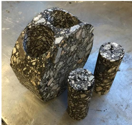
Figure 3.4 Two small specimens produced from one field core
