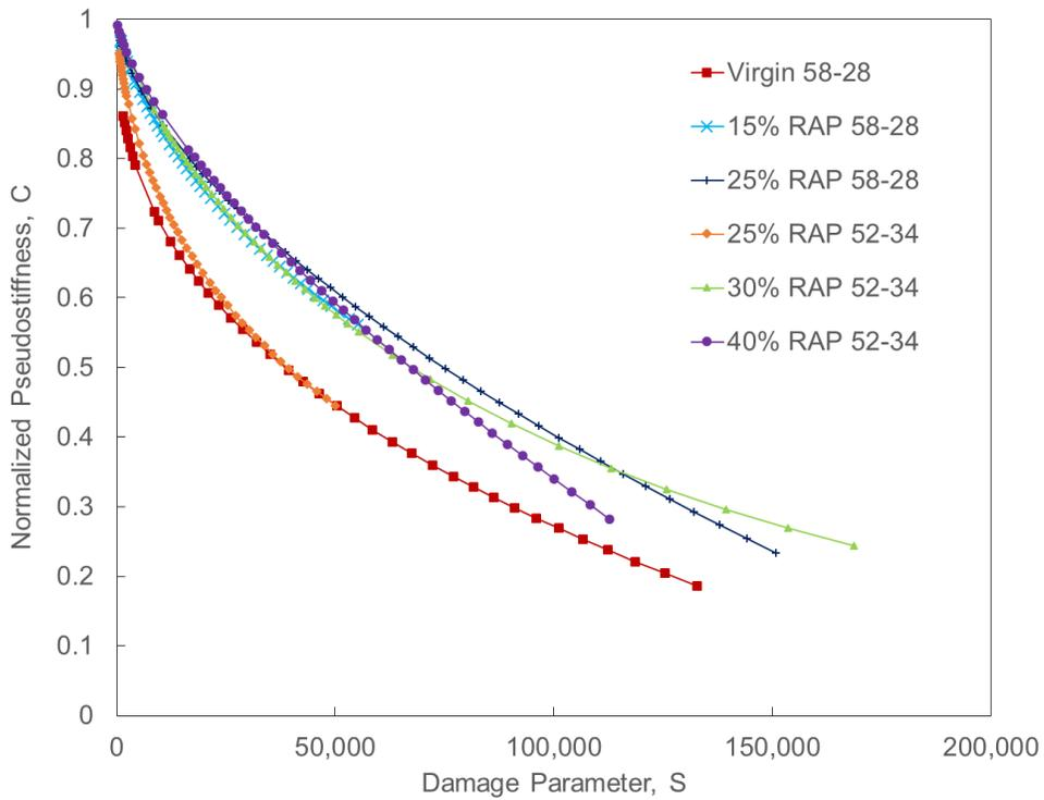
Figure 3.32 Damage Characteristic Curves for PMLC Specimens
