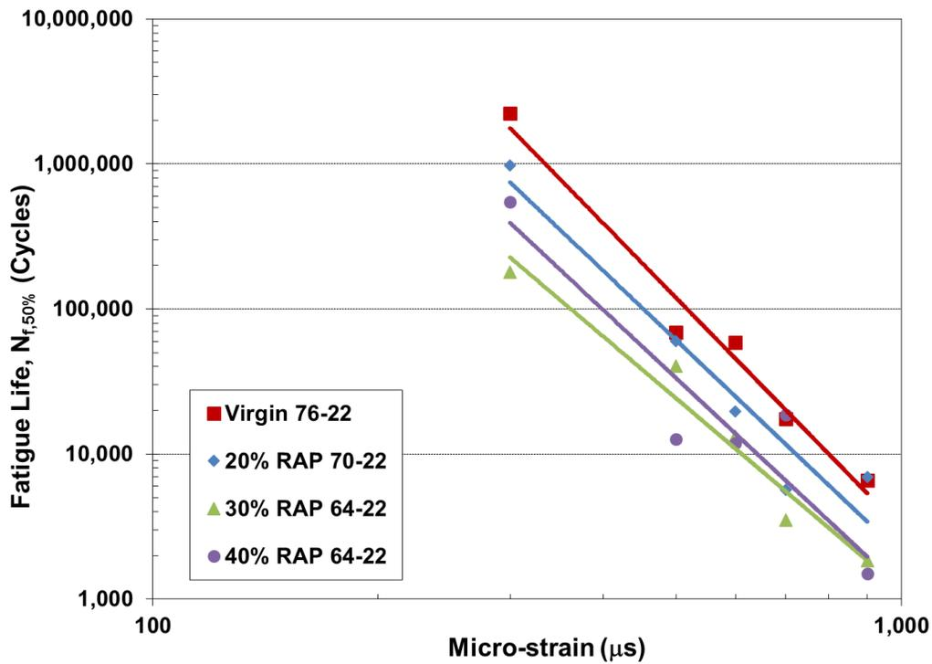
Figure 4.6 Flexural Beam Fatigue Test Results for Virginia RAP Mixtures
