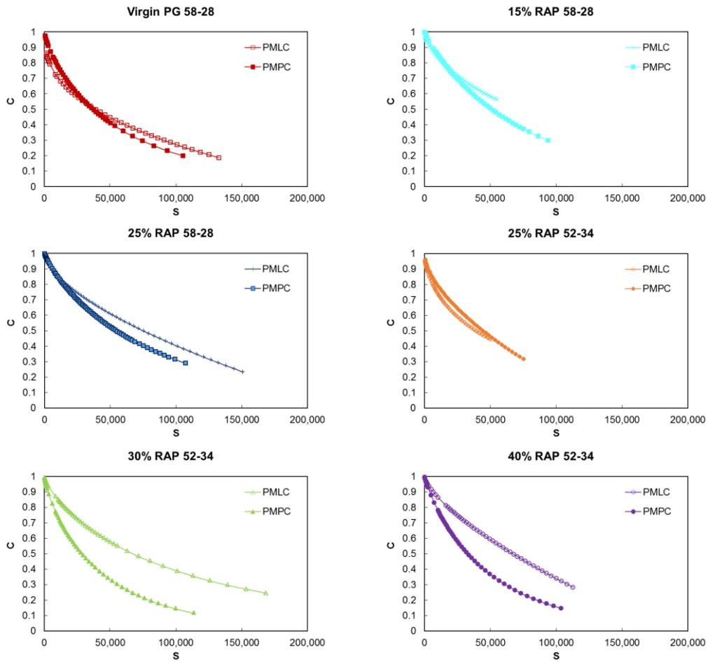
Figure 3.35 Comparison of PMLC and PMPC damage characteristic curves for each mixture
