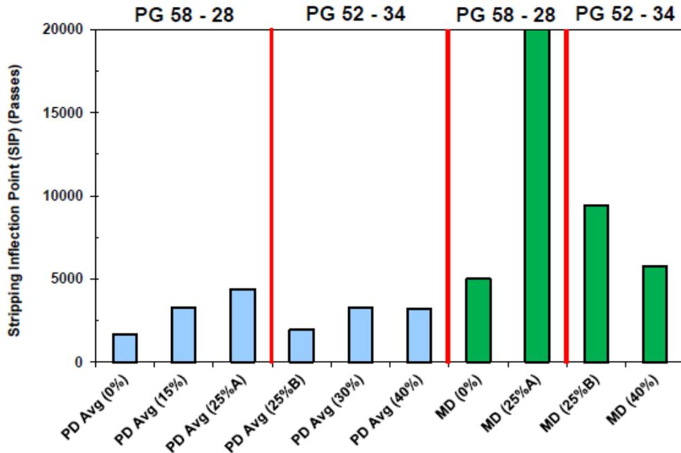
Figure 3.43 Stripping Inflection Point for PMPC (PD) and LMLC (MD) specimens
