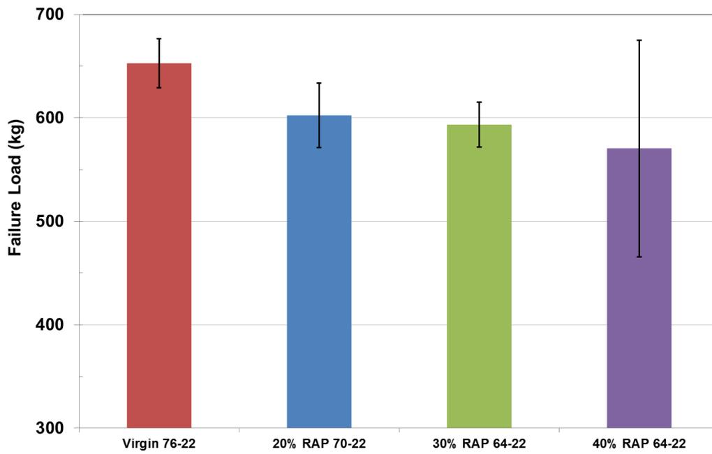
Figure 4.9 TSRST Failure Load for VA PMLC Mixtures
