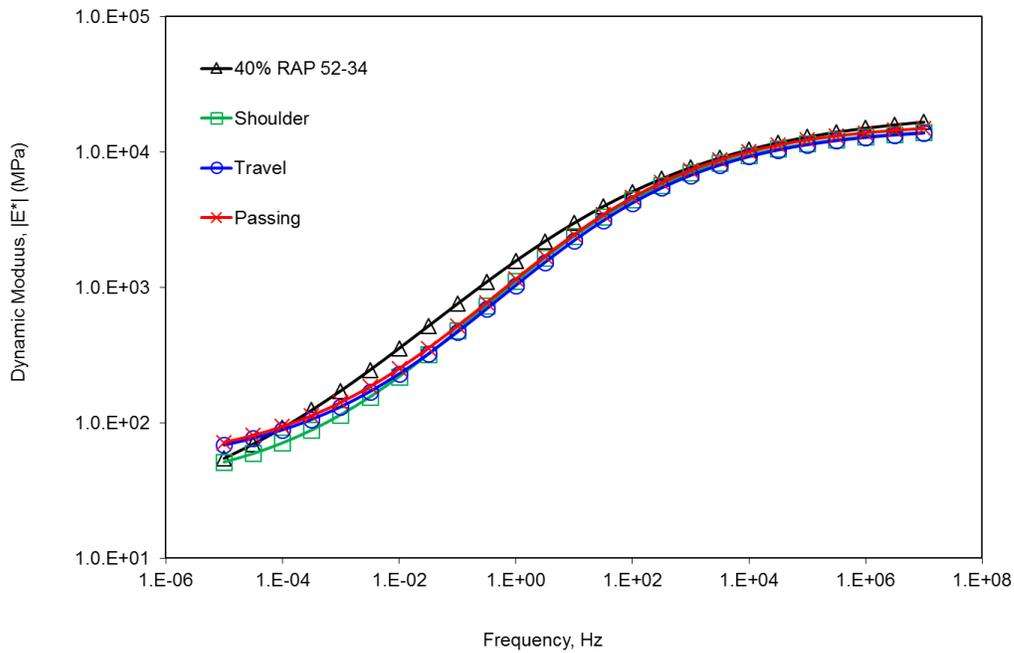
Figure 3.20 40% RAP PG 52-34 Average Dynamic Modulus Curves at 21°C for LMLC and all PMPC Production Days
