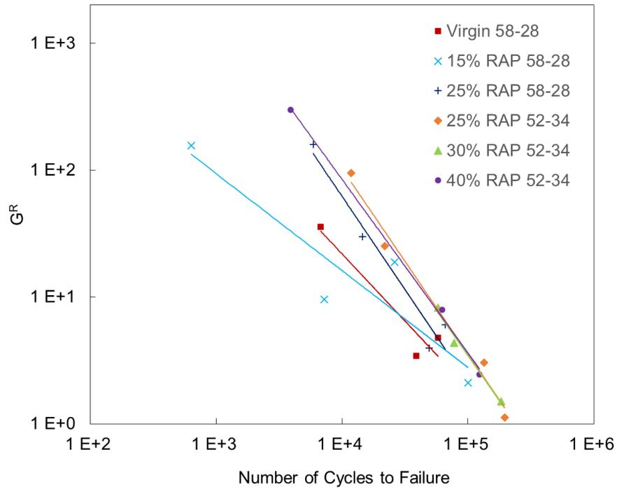
Figure 3.33  $G^R$  versus Number of Cycles to Failure for PMPC Specimens
