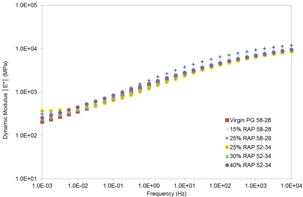
Figure 3.21 Average Dynamic Modulus Master Curves at 21°C for UNH PMPC Specimens
