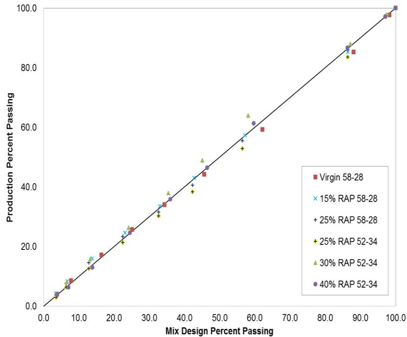
Figure 3.3 Comparison of Production and Mix Design Gradations
