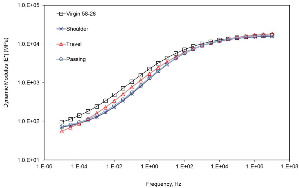
Figure 3.15 Virgin PG 58-28 Average Dynamic Modulus Curves at 21°C for LMLC and all PMPC Production Days
