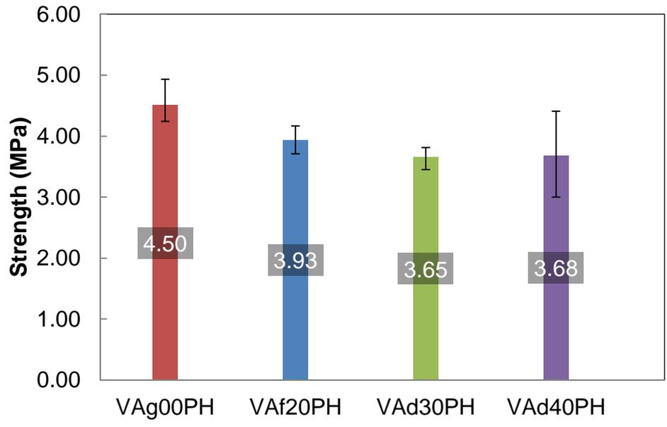
Figure 4.11 Low temperature strength results for VA PMPC Specimens
