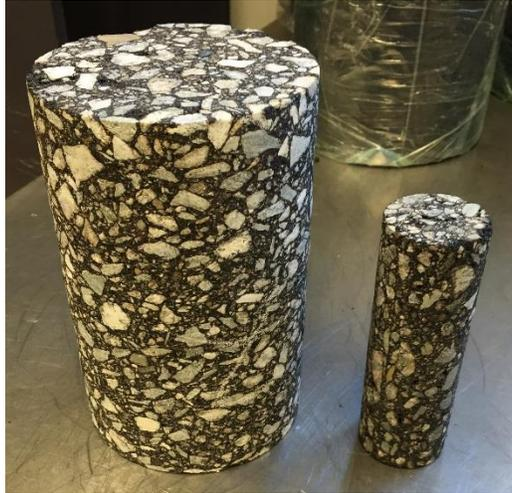
Figure 3.5 Comparison of standard size (left) vs. small geometry specimens (right)
