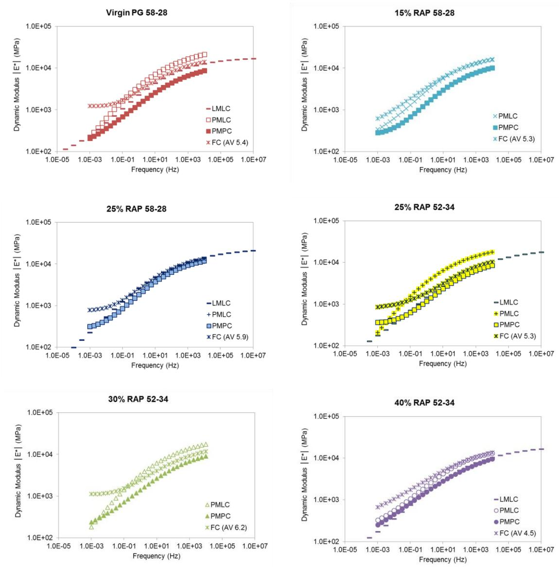
Figure 3.29 Average Dynamic Modulus Master Curves at 21°C for LMLC, PMLC, PMPC, and Field Cores
