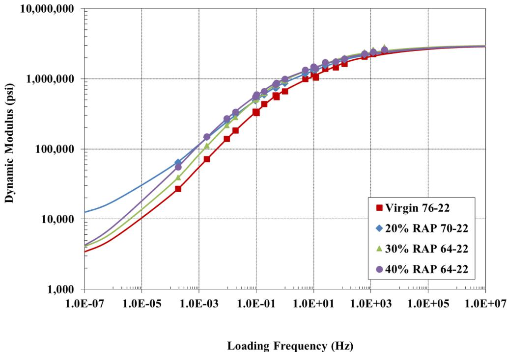
Figure 4.1 Dynamic Modulus Master Curves for VA PMLC Specimens
