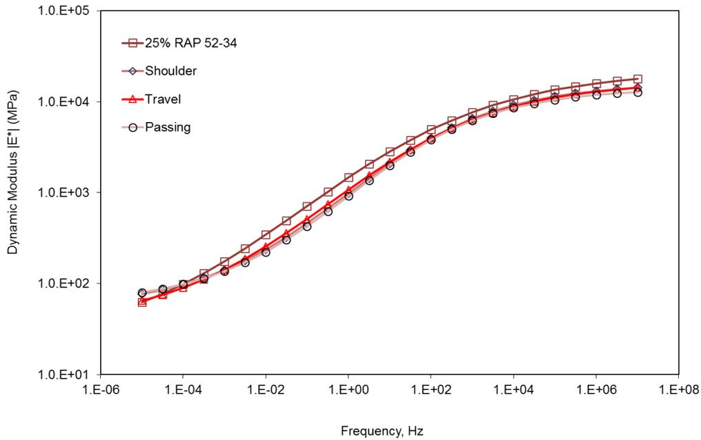
Figure 3.18 25% RAP PG 52-34 Average Dynamic Modulus Curves at 21°C for LMLC and all PMPC Production Days
