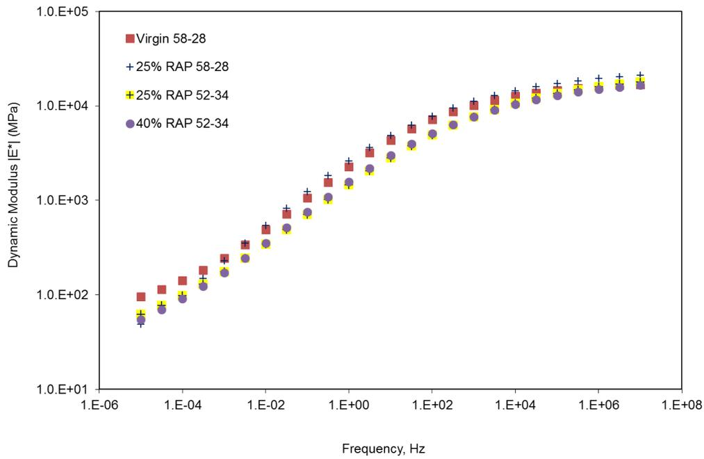
Figure 3.11 Average Master Curves at 21°C for LMLC Specimens
