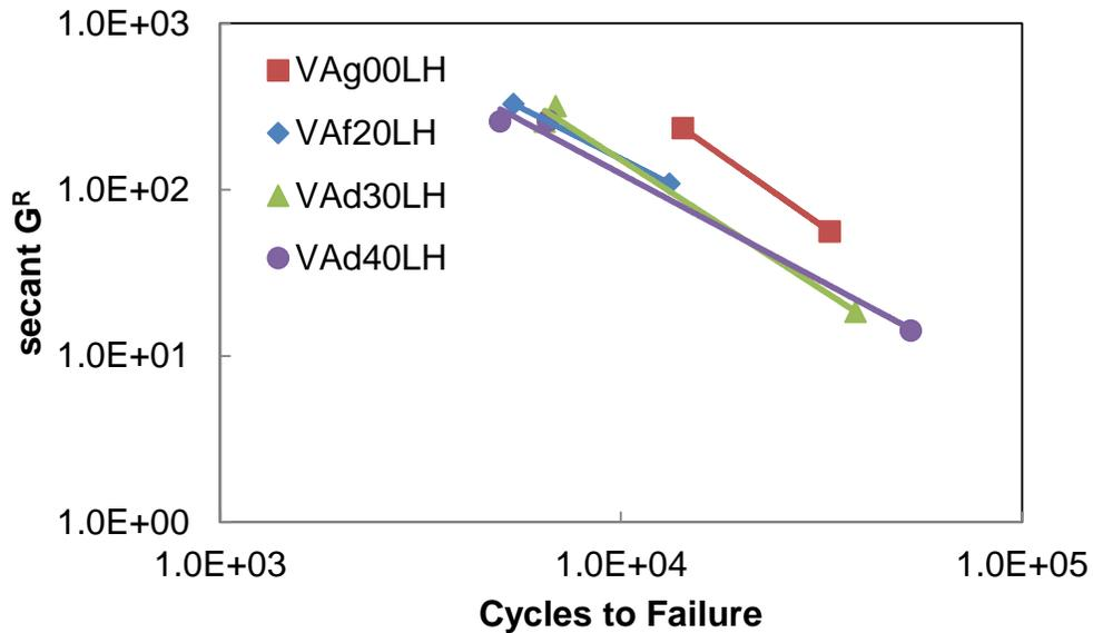
Figure 4.5 Failure Criterion for VA mixtures using secant- $G^R$  method
