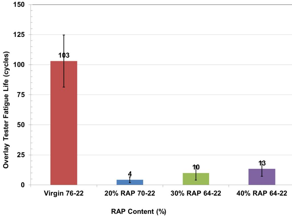
Figure 4.7 Overlay Tester Results for Virginia Mixtures
