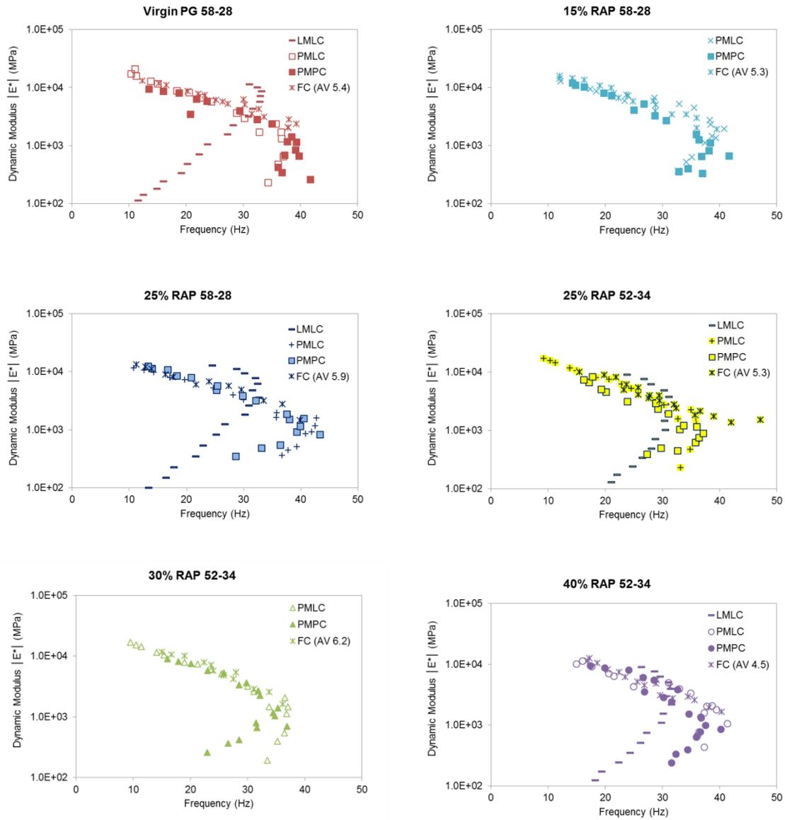
Figure 3.30 Average Black Space Curves for LMLC, PMLC, PMPC, and Field Cores
