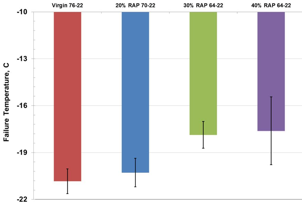
Figure 4.8 TSRST Failure Temperature for VA PMLC Mixtures
