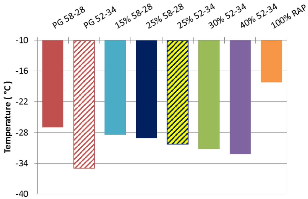
Figure 3.8 Critical Cracking Temperature for Virgin and Extracted and Recovered Binders
