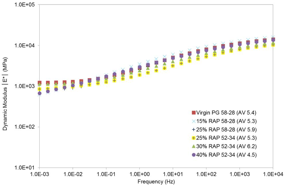
Figure 3.25 Average Dynamic Modulus Master Curves at 21°C for Field Cores
