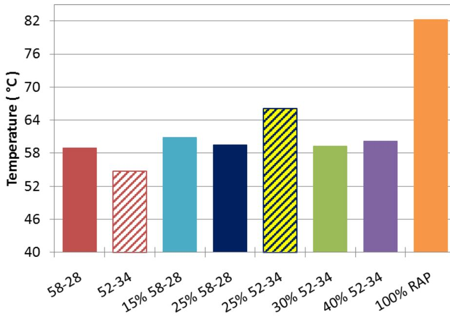
Figure 3.6 Continuous High Temperature Grade for Virgin and Extracted and Recovered Binders
