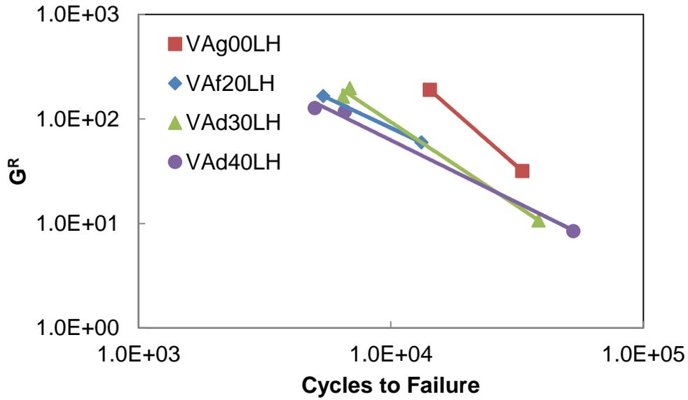
Figure 4.4 Failure Criterion for VA mixtures using  $G^R$  method
