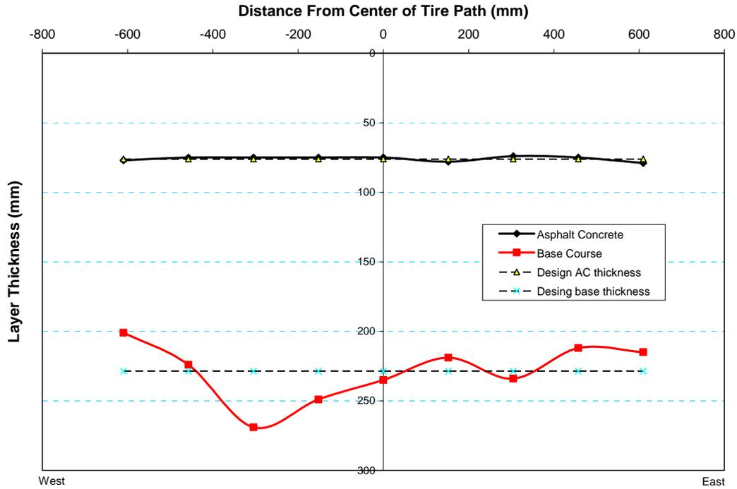
**Figure 40. Layer thickness measurements across Test Window C6.**
