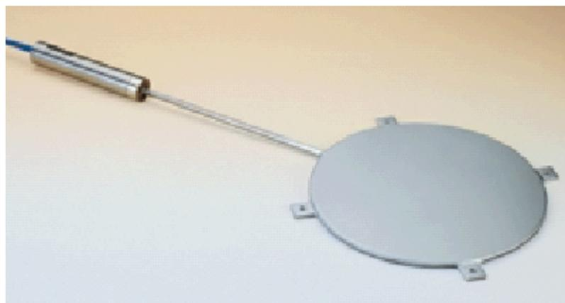
*Figure 11. Geokon® stress cell used in the base course and subgrade.*
