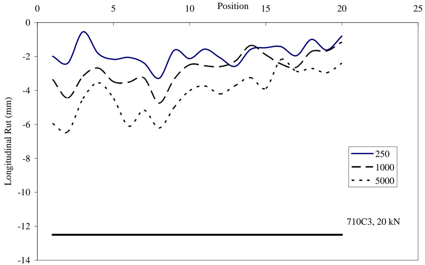
Figure 19. Longitudinal progression of surface rutting in Test Window C3.
