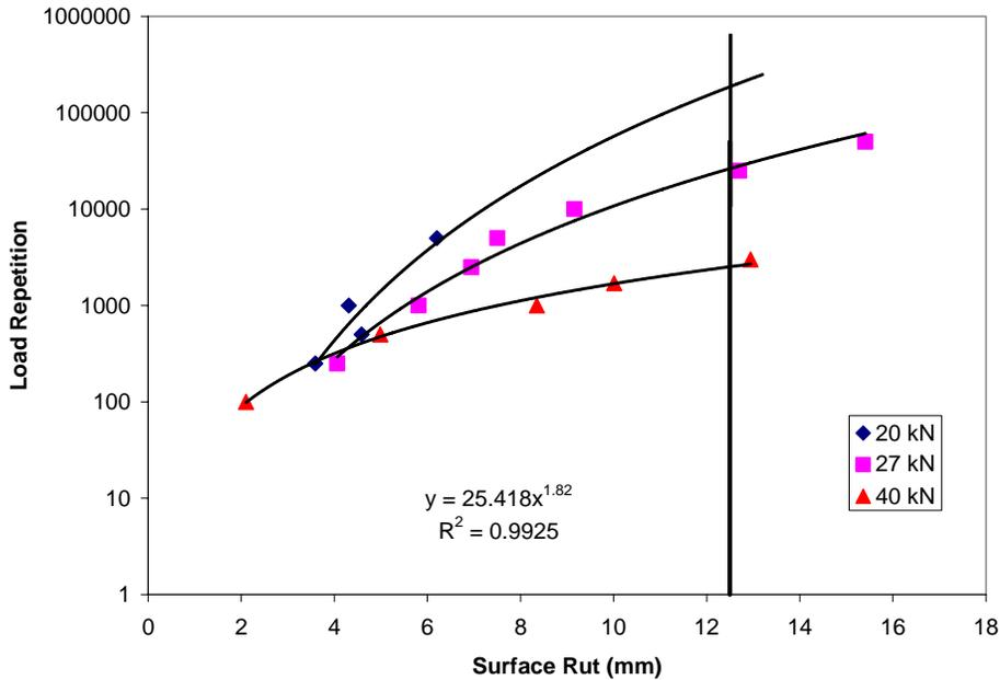
Figure 24 Load repetitions as a function of rut depth.
