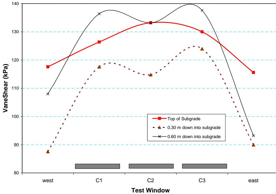
Figure 33. Vane shear measurements in the upper subgrade in the south trench.
