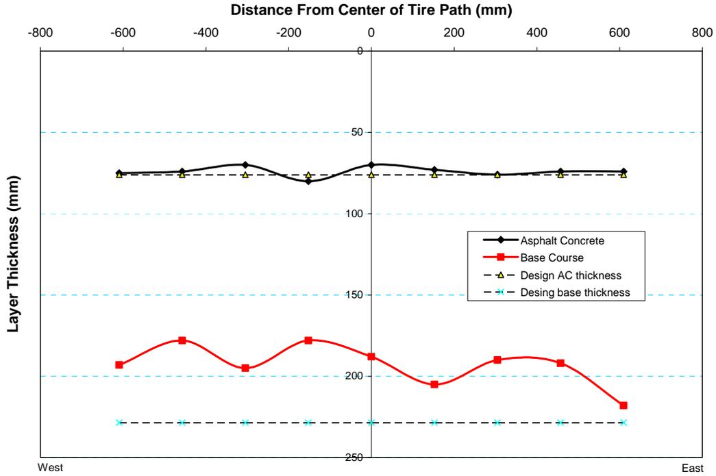
Figure 38. Layer thickness measurements across Test Window C4.
