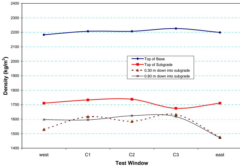
Figure 31. Density measurements in the base and upper subgrade in the south trench.
