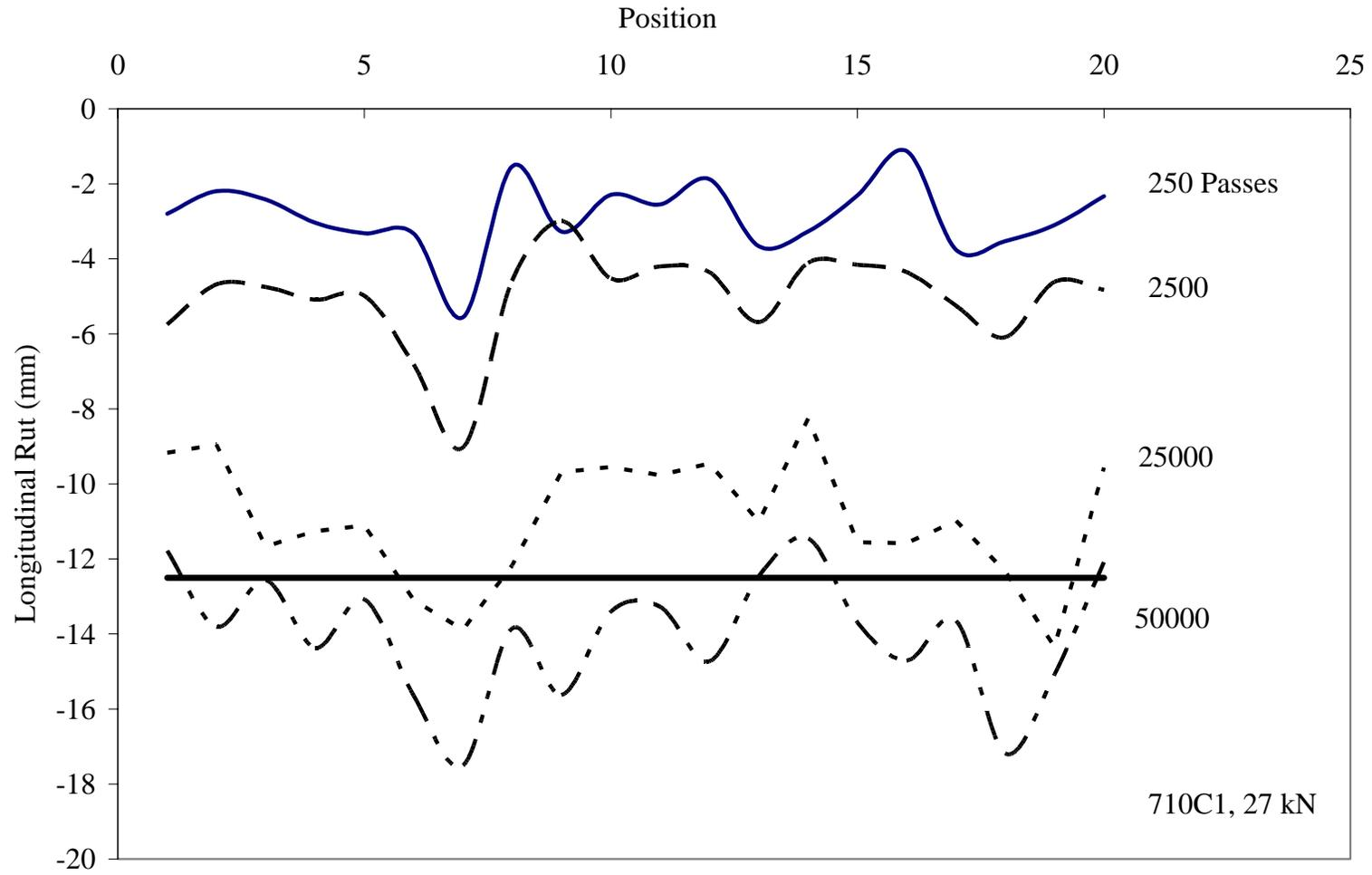
Figure 17. Longitudinal progression of surface rutting in Test Window C1.
