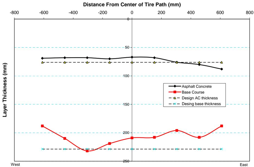
Figure 35. Layer thickness measurements across Test Window C1.
