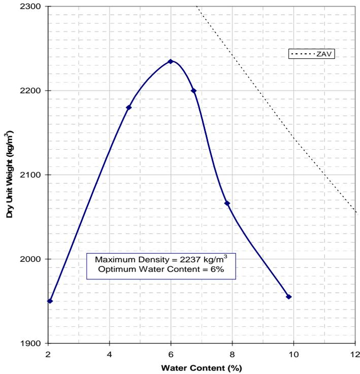
**Figure 4. Base course modified Proctor test result.**
