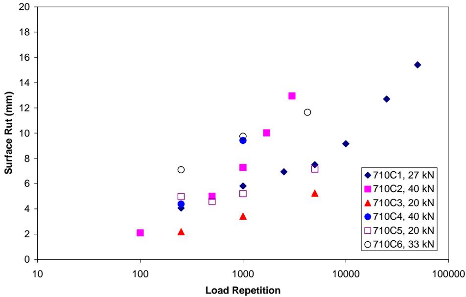
**Figure 23. Rut depth progressions as function of load repetitions.**
