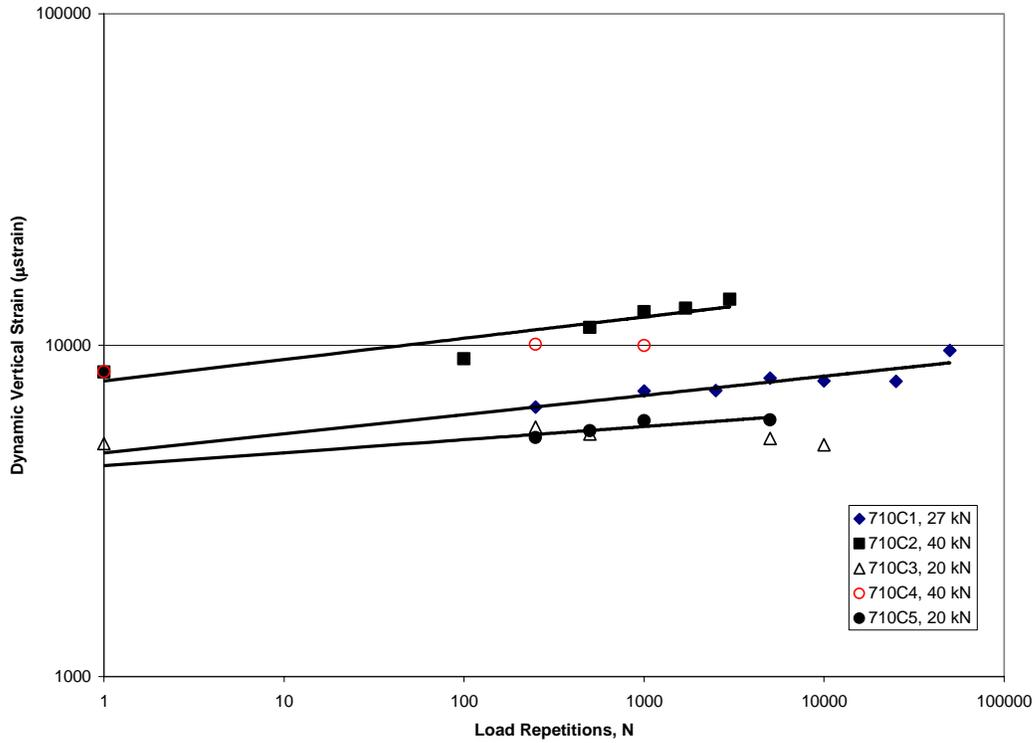
Figure 26. Peak dynamic vertical strains of subgrade as function of load repetitions
