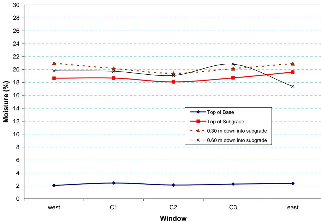
**Figure 29. Moisture content in the base and upper subgrade in the south trench.**
