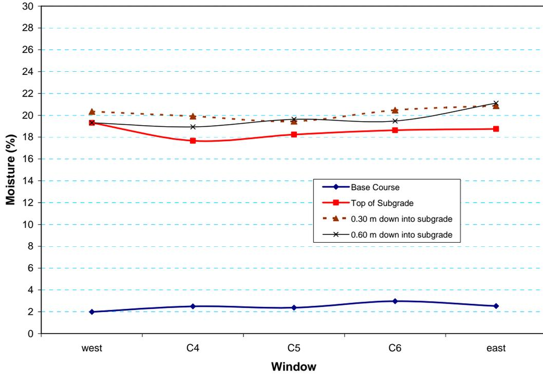
Figure 30. Moisture content in the base and upper subgrade in the north trench.
