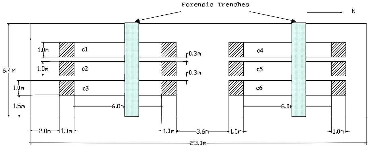
**Figure 27. Location of the forensic trenches in Test Section 710**
