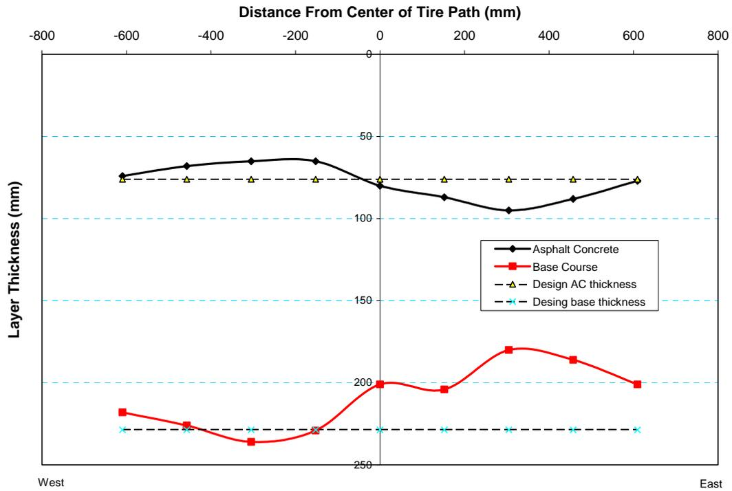
Figure 39. Layer thickness measurements across Test Window C5.
