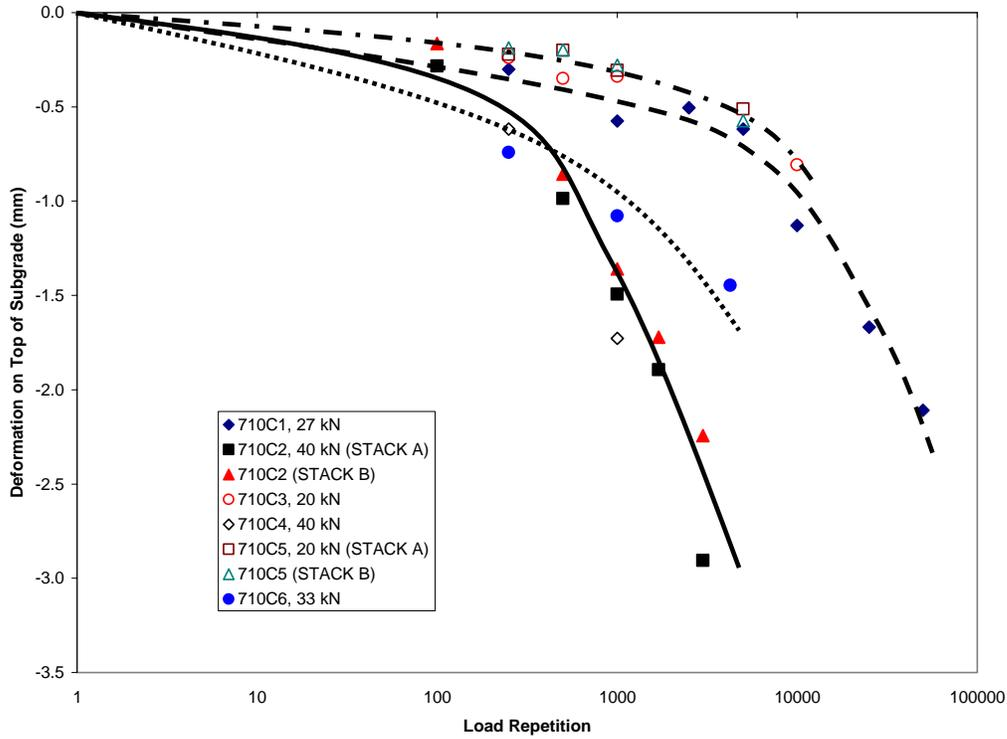
*Figure 25. Permanent deformation at 76 mm below the top of subgrade layer*
