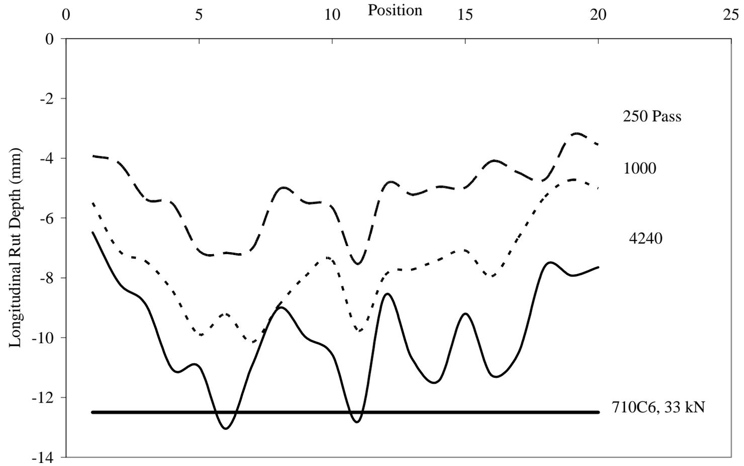
Figure 22. Longitudinal progression of surface rutting in Test Window C6.
