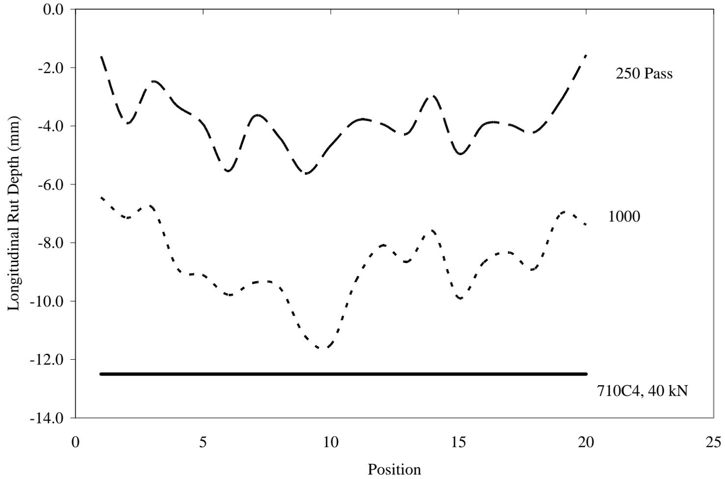
Figure 20. Longitudinal progression of surface rutting in Test Window C4.
