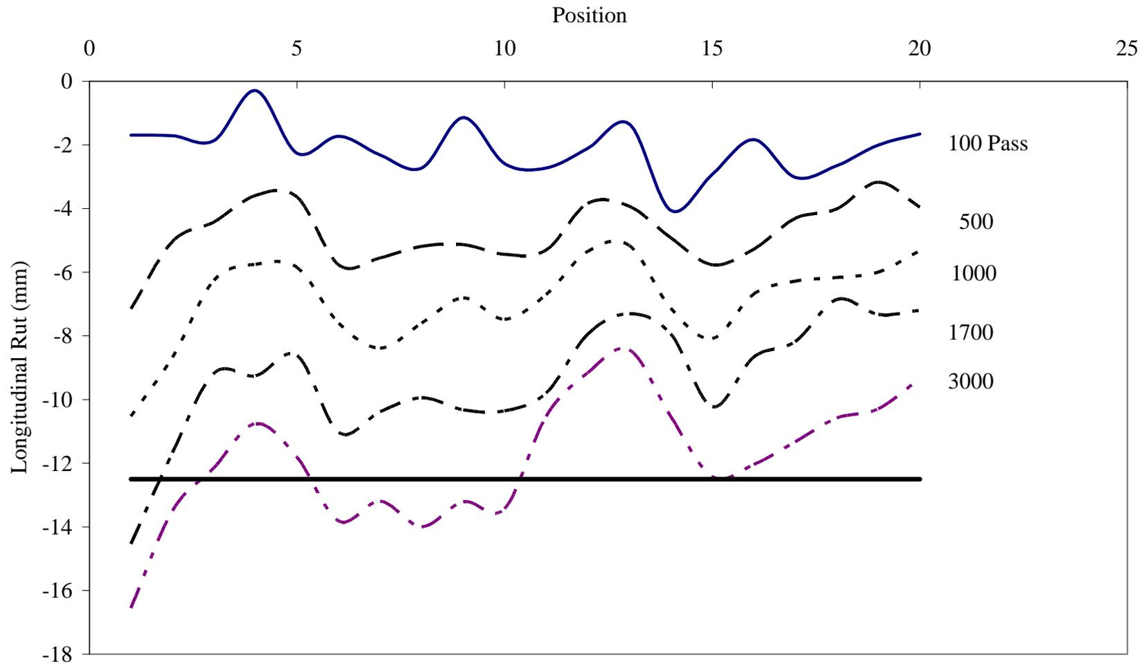
Figure 18. Longitudinal progression of surface rutting in Test Window C2.
