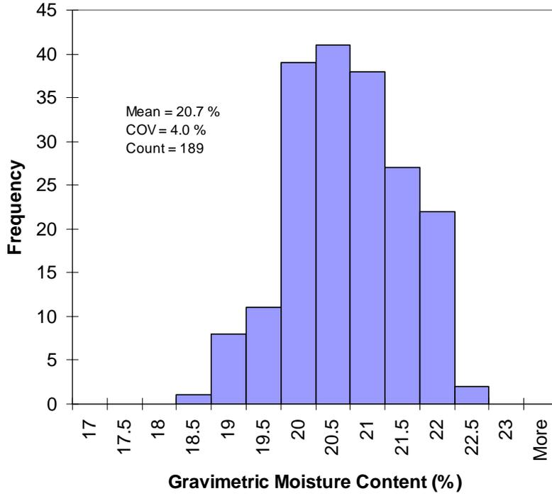
*Figure 5. Subgrade moisture content.*
