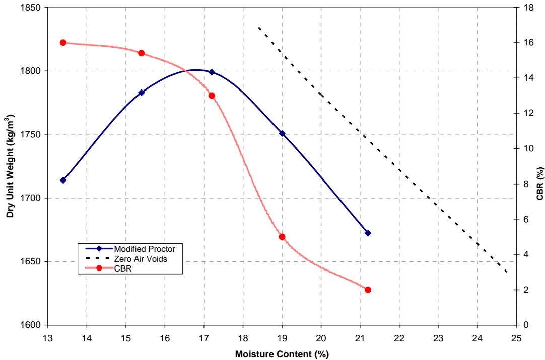
**Figure 3. Modified Proctor and CBR test results for the subgrade soil**
