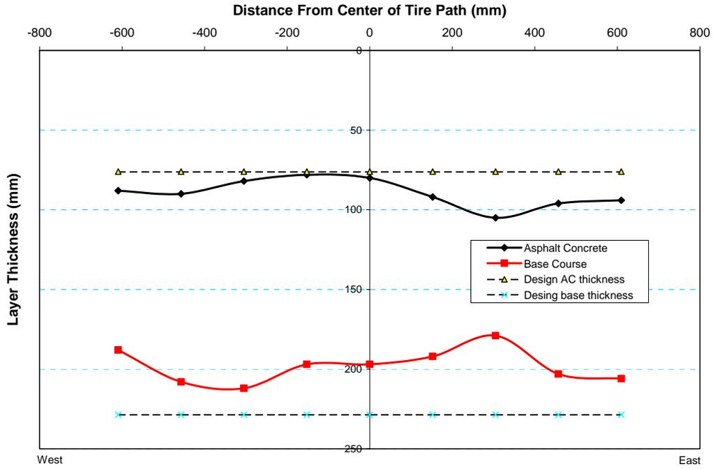
Figure 36. Layer thickness measurements across Test Window C2.
