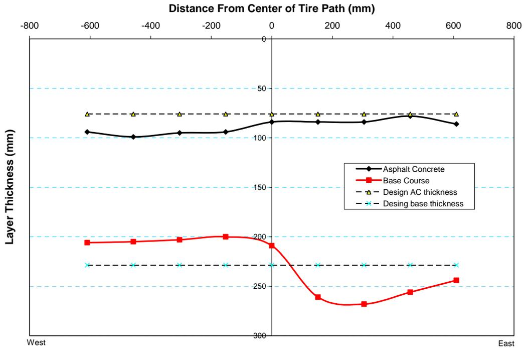
Figure 37. Layer thickness measurements across Test Window C3.
