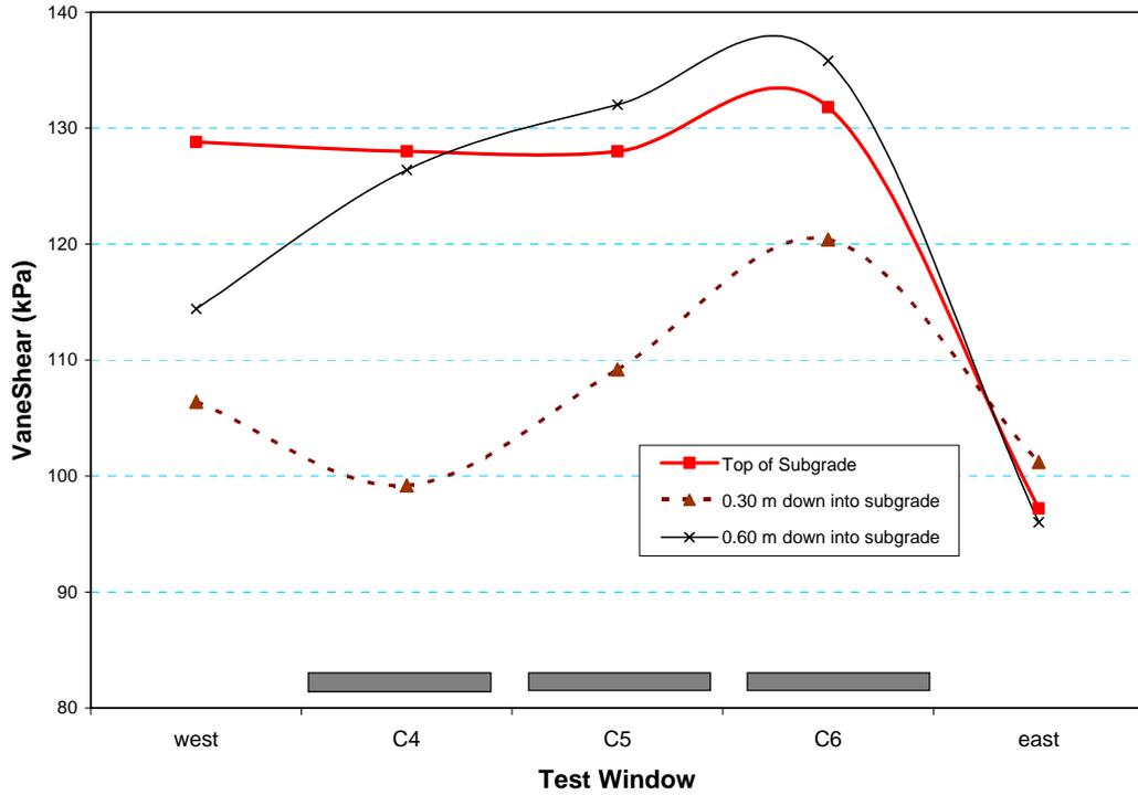
Figure 34. Vane shear measurements in the upper subgrade in the north trench.
