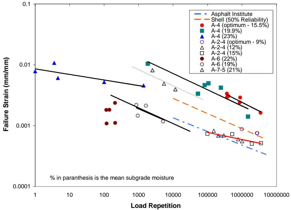
*Figure 41. Effect of soil type on the subgrade failure criterion*
