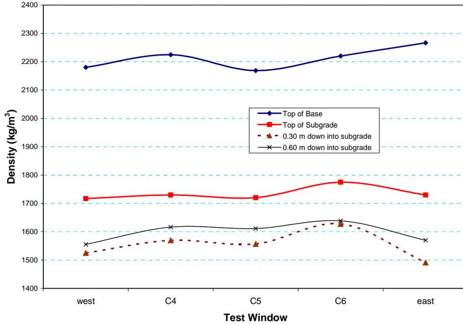
Figure 32. Density measurements in the base and upper subgrade in the north trench.
