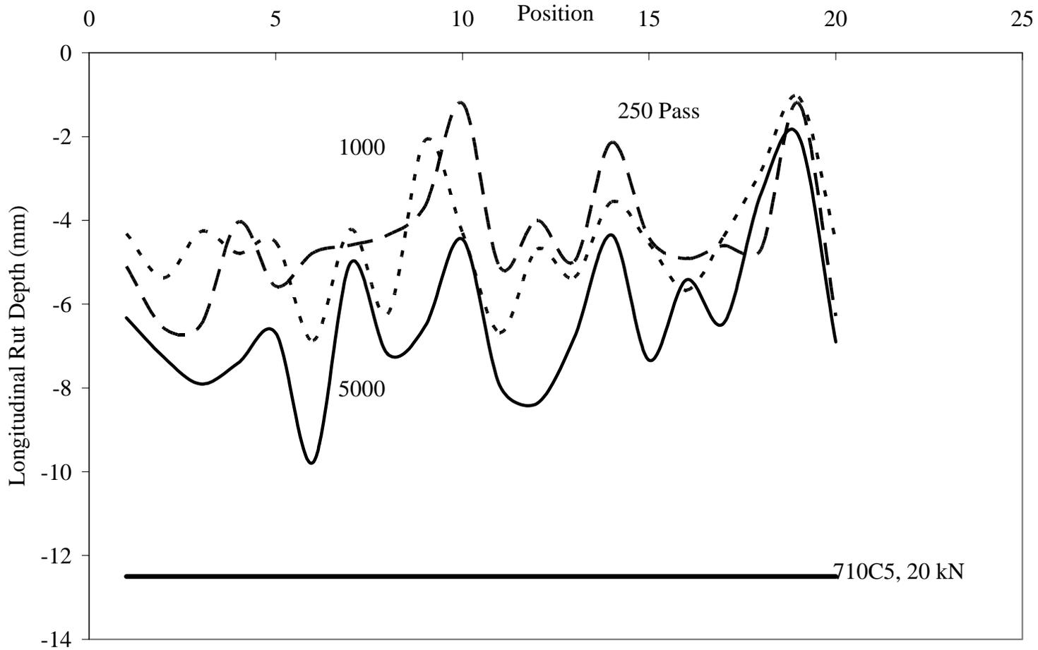
Figure 21. Longitudinal progression of surface rutting in Test Window C5.
