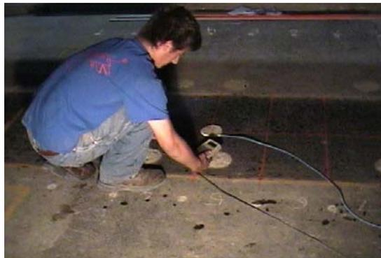
**Figure 16. Measuring displacement between the AC surface and the top of the base course.**
