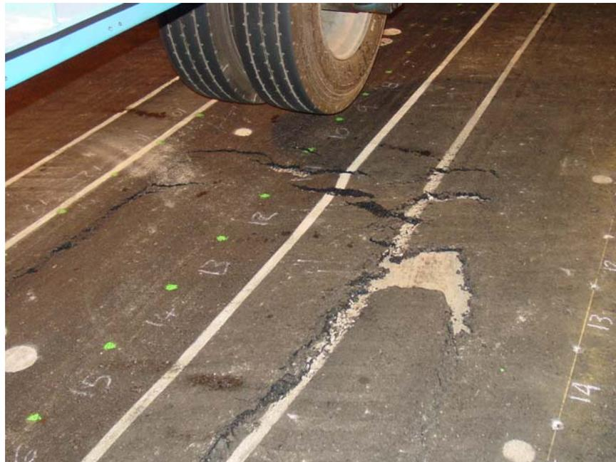
Figure 25. Test Window 709c5 at the end of HVS traffic.
