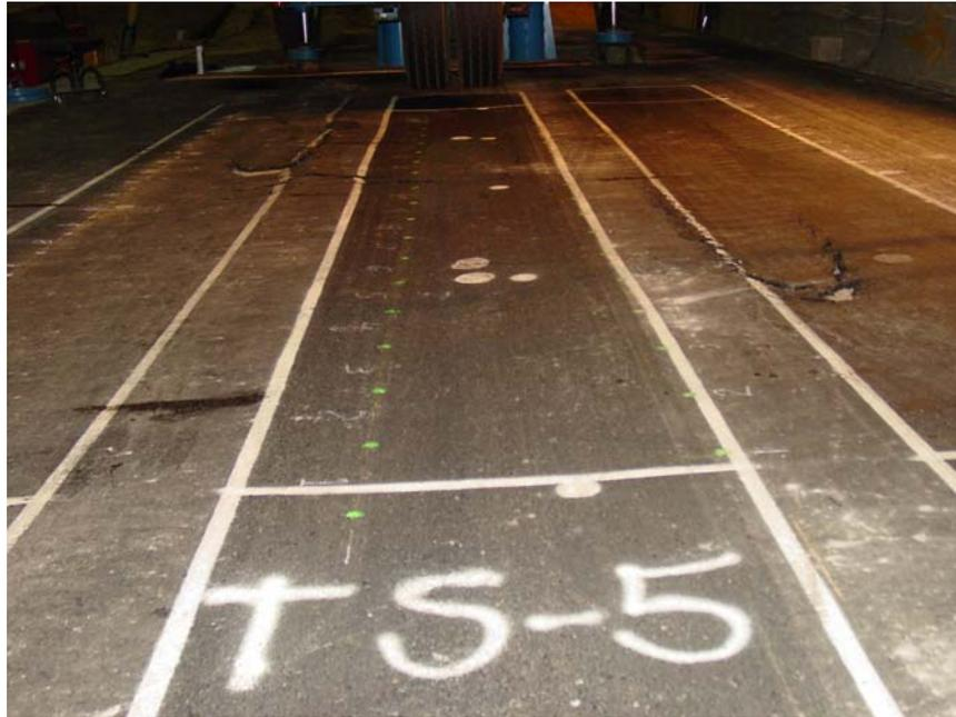
Figure 24. Damage to Test Windows 709c5 caused by neighboring test windows.
