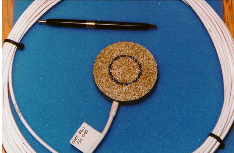
*Figure 10. Dynatest® stress cell used in the subgrade.*
