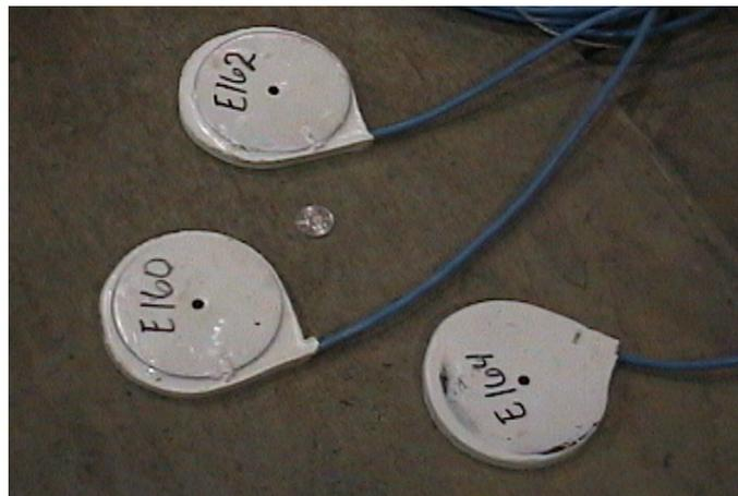
*Figure 9. Emu coils in a co-planar arrangement to measure longitudinal and transverse deformations. A US 25-cent coin is included for scale reference.*
