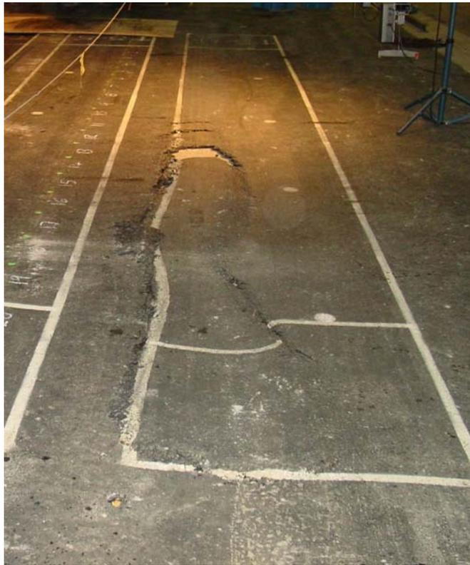
Figure 23. Test Window 709c4 at the end of HVS traffic.
