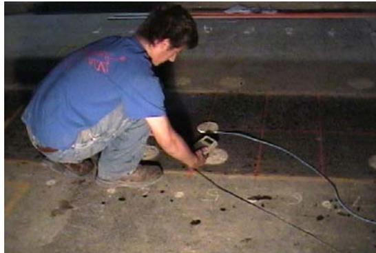
**Figure 16. Measuring vertical deformation between the AC surface and the top of the base course.**
